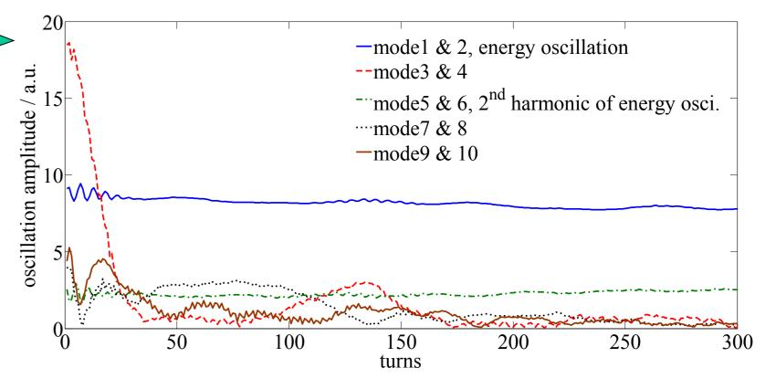
detailed evolution of the modes obtained by using the right-singular vectors of the motion matrix
