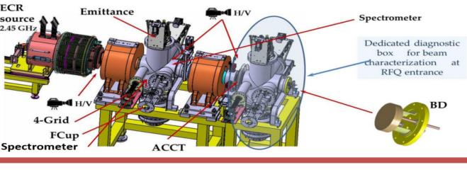
High beam space charge: To minimize the emittance growth, LEBT length minimized to 2.05 m
