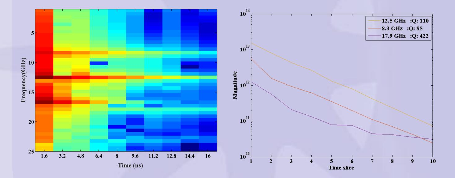
Are the decays of the resonances following the expected exponential trend, and are the resulting Q values believable? code helps in the extracting of trends and the detailed study of specific aspects of a structures behaviour.
