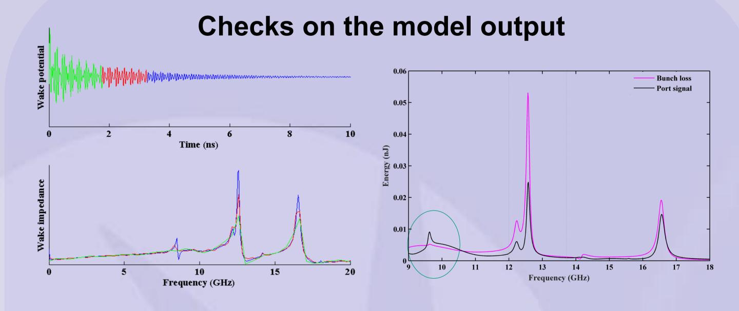
**Truncation of the time data** leads to errors in the wake impedance.
