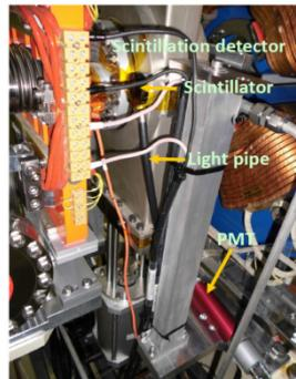
Installation location of scintillation detector.
