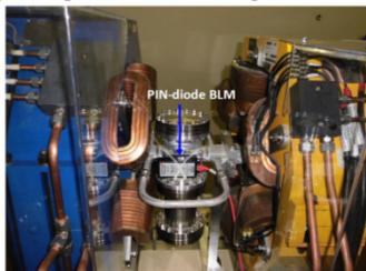
(b) The setup of a PIN-diode BLM.
