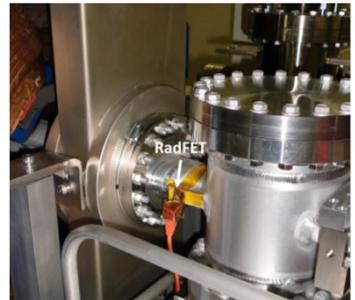
(d) RadFETs are installed in the inside-wall chamber of the storage ring.
