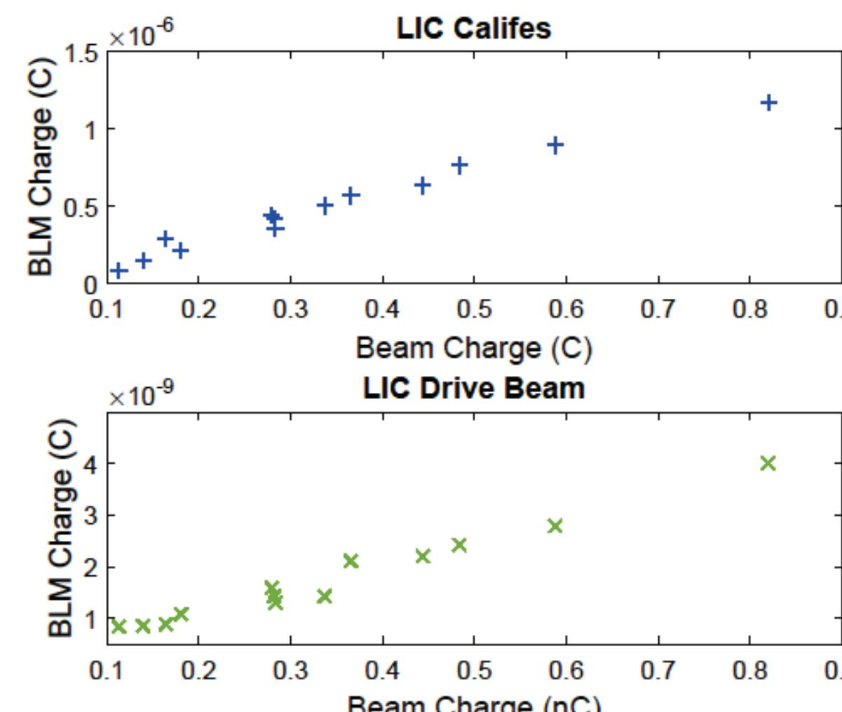
Main Beam → Drive Beam crosstalk smaller than 1%
