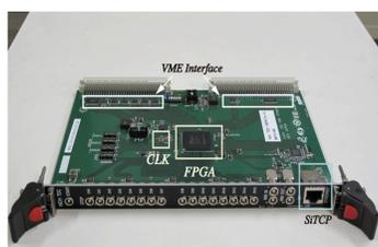
Fig.2: Developed VME/FPGA-based TDC module.
