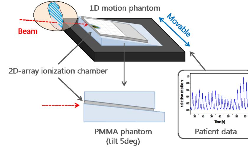
In the additional QA for moving target irradiation, we place a 2D ionization chamber (Octavius Detector 729 XDR, PTW Freiburg, Germany) on the PMMA plate tilted with respect to the beam axis. The PMMA plate is set on the stage of the moving phantom (model 008PL, CIRS). The moving phantom can be moved in the transverse direction according to the patient data.
