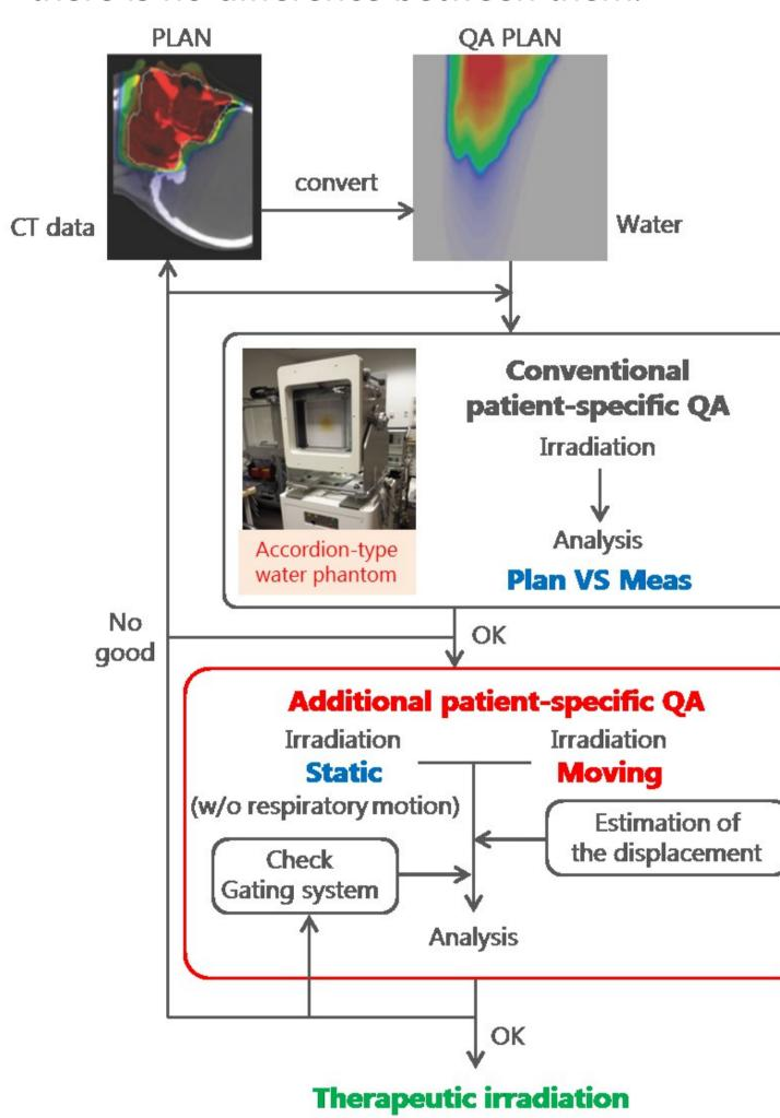
Measurement setup in an additional QA
