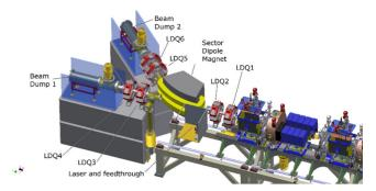
Figure 5: CAD model of the laserwire lattice showing the six quadrupoles (LDQn), the  $45^{\circ}$  sector-bend dipole magnet, the laser feedthrough and the beam dumps.
