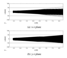
Figure 7: Particle trajectories with the dipole switched off.
