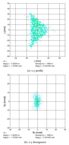
Figure 10: Beam at the entrance face of dump 2.
