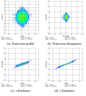
Figure 12: Phase space distribution of the beam of neutrals at the detector location.
