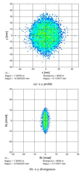
Figure 8: Beam at the entrance face of dump 1.
