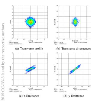
$\bigcirc$  Figure 11: Phase space distrbution of the stripped beam used as the input beam for tracking neutrals to the detector.
