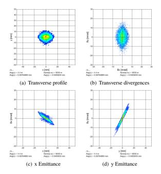
Figure 6: Phase space distrbution of the input beam used in the tracking simulations.
