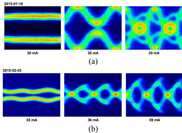
Figure 11: Longitudinal instability behavior of the stored beam observed by streak camera in TPS commissioning before amplitude feedback loop problem of RF system was identified. Both cases with difference chromaticity setting. (a) Stored beam current increase from 20 mA to 30 mA, (b) from 35 mA to 59 mA. Vertical time scale = 700 ps, horizontal time scale = 1 ms.
