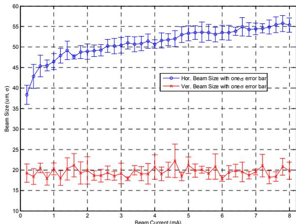
Figure 5: Plot of beam size measurement by X-ray pinhole camera in horizontal and vertical direction versus beam current under single bunch mode.
