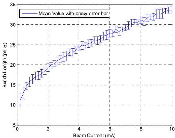
Figure 10: The relative relationship between the beam current and bunch length under the single bunch mode.
