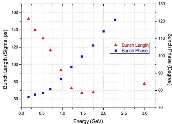
Figure 8: Bunch length and phase variation during the energy ramping process. Bunch length changes around 85 psec, bunch phase change around 45 degree.
