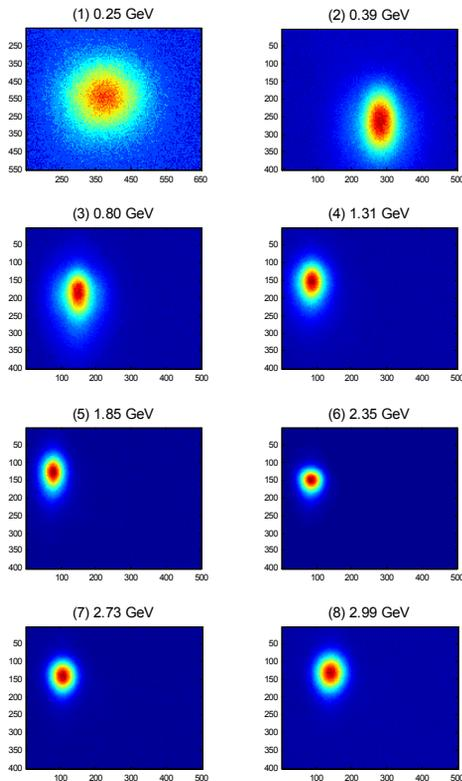
Figure 3: TPS booster synchrotron radiation profiles at varied energy during energy ramping, one pixel corresponding to 9  $\mu\text{m}$ .
