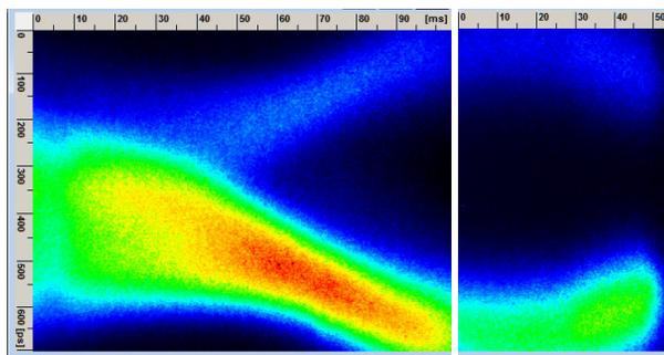
Figure 7: Bunch length as shrink during booster energy ramping observed by streak camera, vertical time scale = 700 ps, time scale for horizontal is millisecond.
