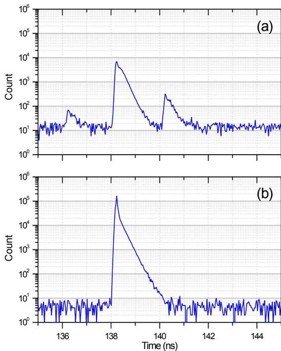
Figure 13: Single bunch purity measurement by TCSPC technique (5 sec accumulation), (a) before and (b) after bunch cleaning applied.
