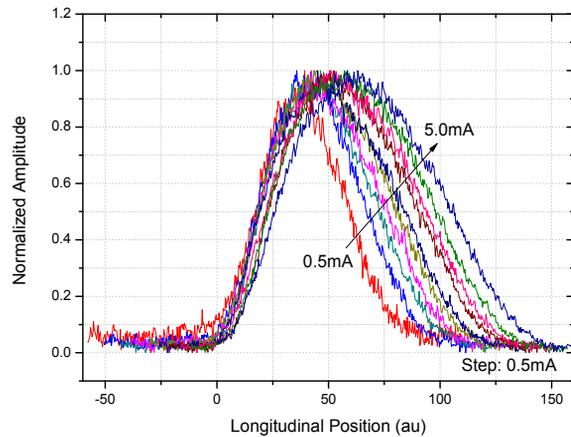
Figure 9: Single bunch profile distortion as function of beam current.
