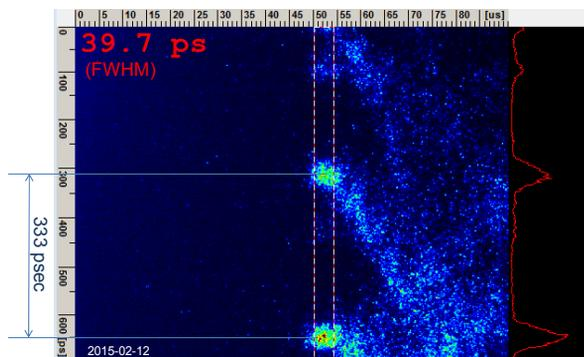
Figure 6: Injection point of at booster under single bunch mode, the bunch length ~17 ps ( $1 \sigma$ ), vertical time scale = 700 ps, horizontal time scale = 90  $\mu$ s.
