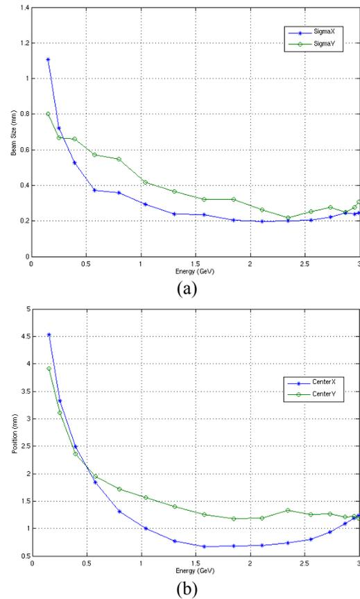
Figure 4: SRM measured of booster synchrotron during energy ramping from 150 MeV to 3 GeV, the variation of (a) beam size and (b) beam center position.
