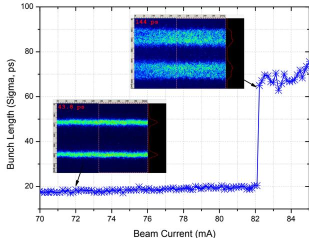
Figure 12: Longitudinal instability onset at 82 mA is indicated by the trace width of the streak camera increase in multi-bunch mode. Bunch length can measure before by the trace width below instability threshold. However, it failed after instability appeared.
