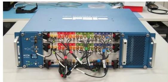
Figure 9: Modular BPM unit, with two cavity BPM RFFEs (top) and FPGA carrier board with two ADC mezzanines (bottom).
