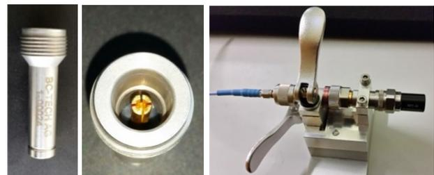
Figure 2: SwissFEL RF feedthrough (left, middle) with test adapter (right) that uses a standard APCN-7 adapter and 50 $\Omega$  broadband load.
