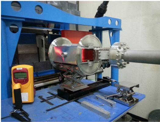
Figure 11: Picture of beam test set-up with moving stage after beam window of test linac.
