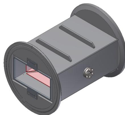
Figure 2: Linear-cut beam position monitor in KHIMA synchrotron.
