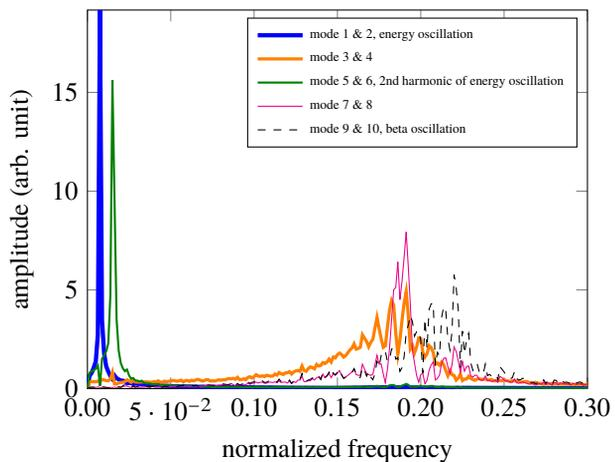
Figure 6: Spectra of the modes separated by SVD.
