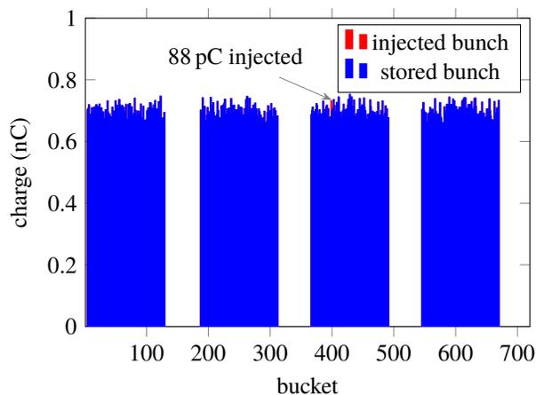
Figure 1: Filling patterns before and after an injection.
