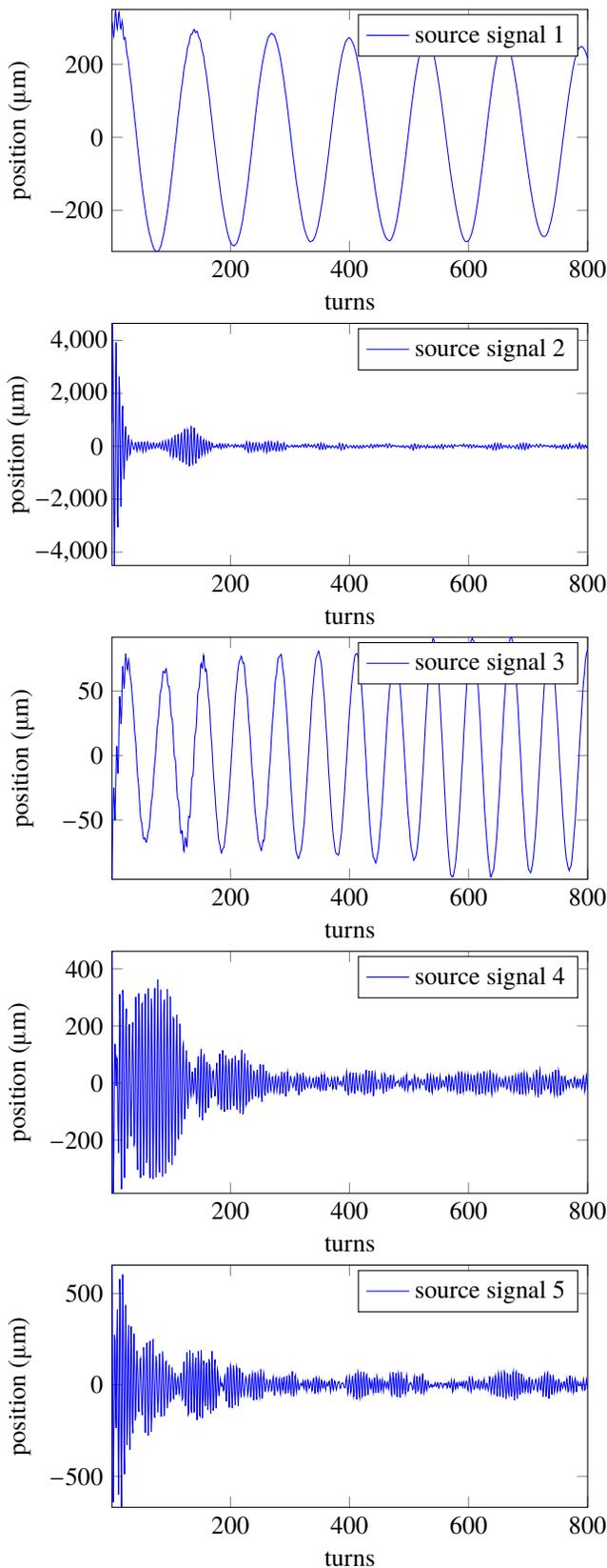
Figure 3: Sources separated from the motion matrix using ICA. The signals 1 and 3 are energy oscillation related and do not decay with time.
