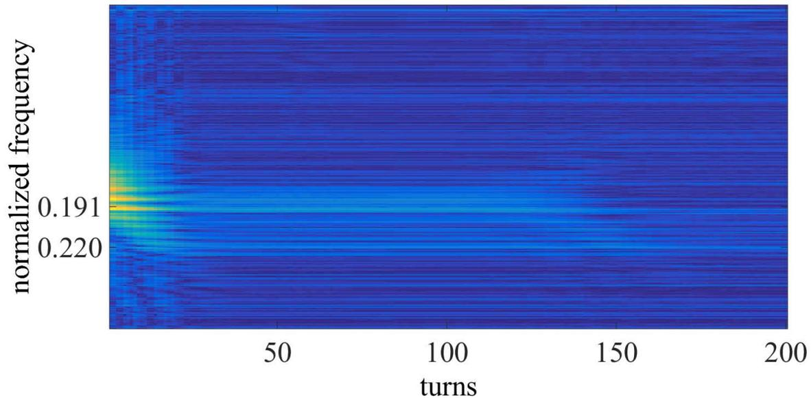
Figure 7: Spectra waterfall of the motion of the injected bunch.
