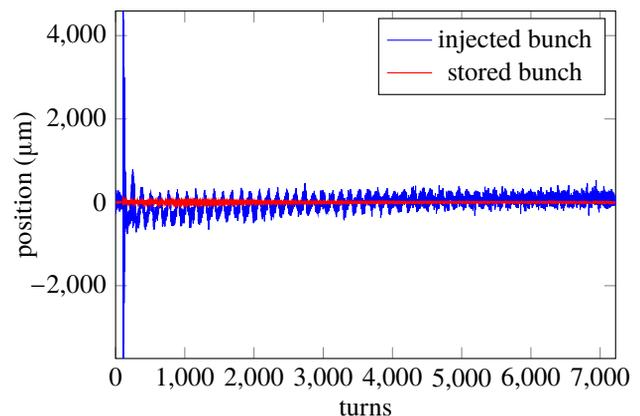
Figure 2: Horizontal positions of the injected bunch separated from the stored one.
