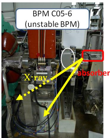
Figure 9: Layout of the BPM C05-6 and the photon absorber
