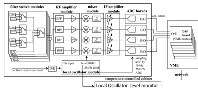
Figure 1: Block diagram of the SPRING-8 BPM circuits.
