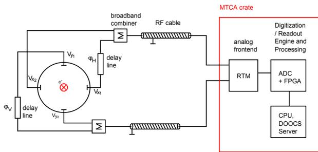
Figure 2: Beam Position Monitor System Overview.
