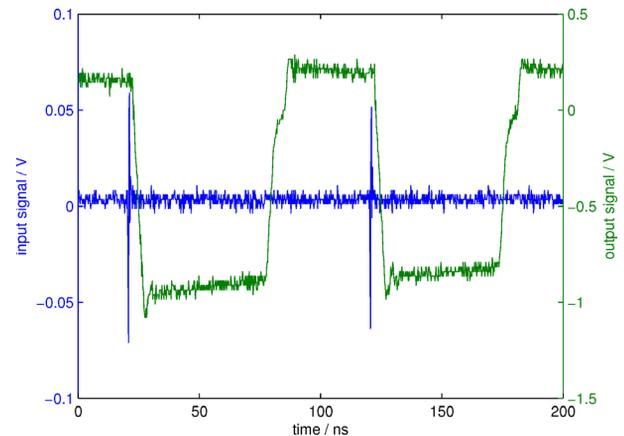
Figure 3: Blue: A typical input signal for the BPM electronics. Green: A typical output signal from the analog front-end before digitization.
