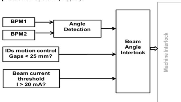
Figure 3: General architecture of the beam angle interlock system.
