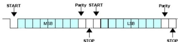
Figure 5: Data protocol over the RS485 transmission line.
