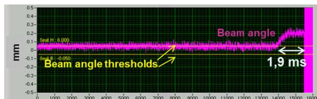
Figure 7: The beam is killed 1.9 ms after the beam angle exceed the threshold.
