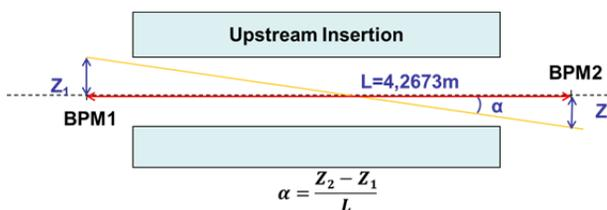
Figure 2: The new beam angle interlock should detect beam angle default between the two BPMs around the upstream insertion device.
