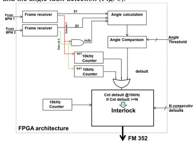
Figure 6: FPGA architecture for the angle detection.
