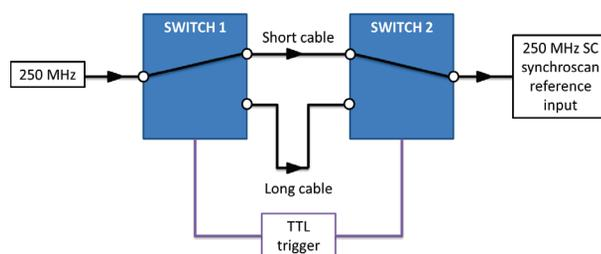
Figure 8: Illustration of the electrical delay introduced using PIN diode switches and cables of different lengths for the fast deflection signal.
