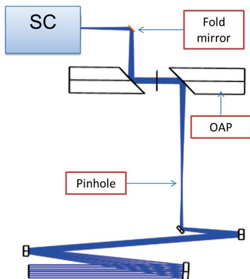
Figure 6: Layout of the upgraded reflective input optics.
