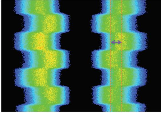
Figure 9: Streak camera calibration image taken in normal user beam where the separation between the dashed red lines is the measured delay used for calibration of the fast timebase. The slow timebase may be calibrated using the period of the square wave.
