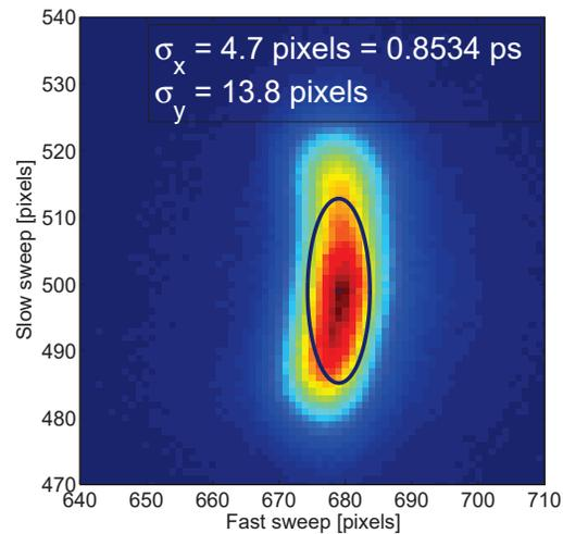
Figure 5: PSF acquired using the previously implemented reflective input optics.
