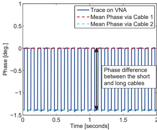
Figure 10: A plot of the 250 MHz VNA trace (blue line) with 10 Hz switching frequency between the short and long cables where the mean phase delays for each cable are shown by the dashed lines.
