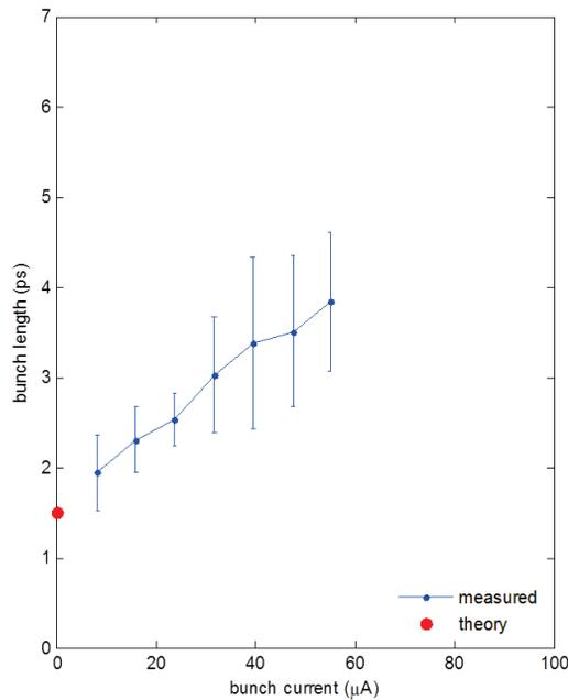
Figure 12: A plot of bunch length at various bunch currents in single bunch low alpha mode at 3.4 MV,  $\alpha = -4.6 \times 10^{-6}$  and  $f_s = 460$  Hz [8]. The error bars indicate the standard deviation over the  $\approx 800$  individual profiles analysed in each streak image.
