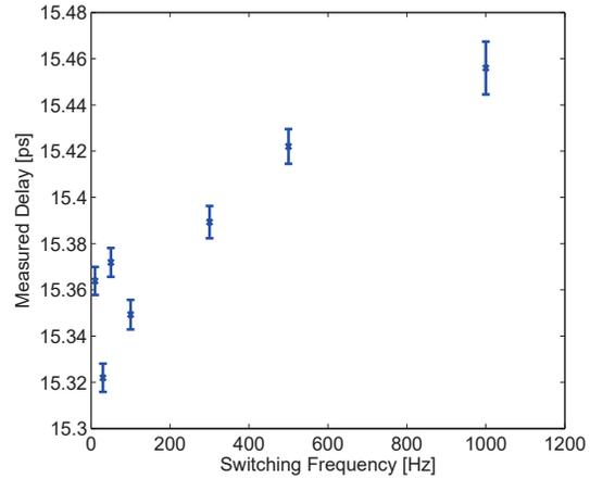
Figure 11: A plot of the measured electrical delay using the VNA for different trigger frequencies provided by the waveform generator. Data points with corresponding standard errors are denoted by crosses and errorbars.
