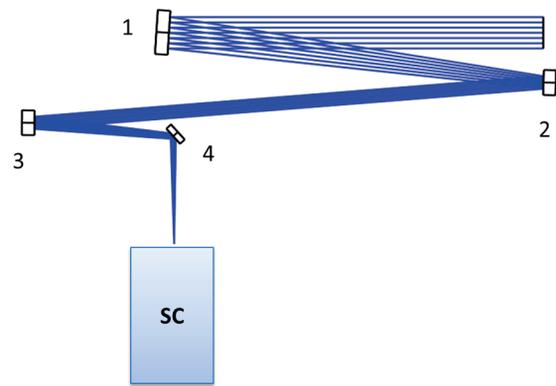
Figure 4: Original reflective input optics where (1) is concave parabolic mirror, (2) is a convex spherical mirror, (3) is a concave spherical mirror and (4) is a flat folding mirror.
