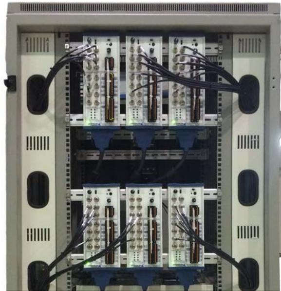
Figure 4: BNC terminal boxes installed on rear rack.
