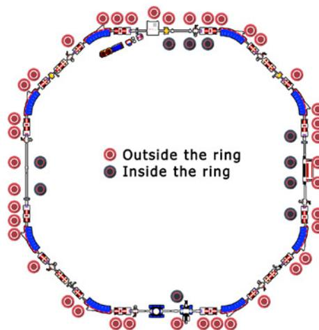
Figure 1: New SPS beam loss monitor positioning layout in storage ring.
