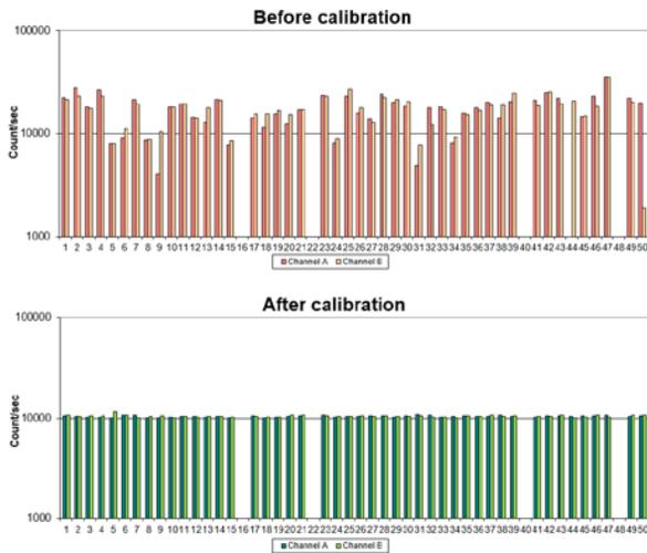
Figure 3: The count rate of BLMs in test mode before and after re-calibration.
