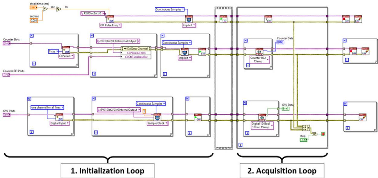
Figure 5: NI LabVIEW DAQmx block diagram.
