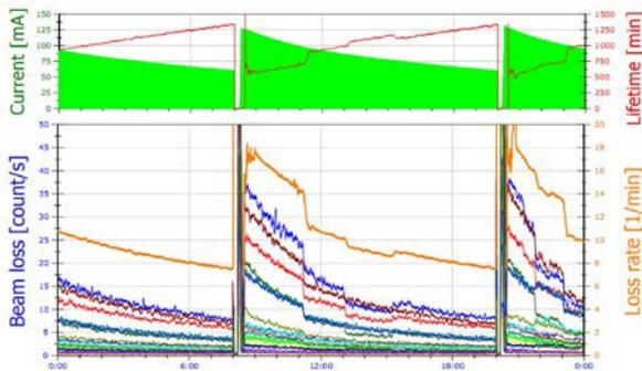
Figure 6: Measured beam loss rate.
