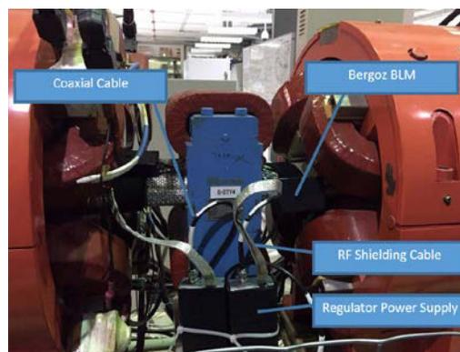
Figure 2: BLMs with RF shielding attached to the vacuum chamber.
