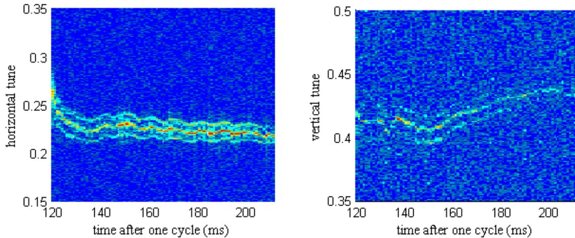
Figure 2: FFT of the signal from BPM showing horizontal tune (left) and vertical tune (right) at the injection point in the booster. Electrons were injected into the booster at 119.5 ms after one cycle trigger.
