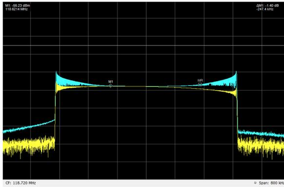
Figure 4: FM signal on spectrocope in real-time mode (yellow) and max hold mode (blue). The center frequency is 118.79 MHz with 500 kHz span.
