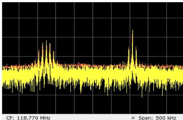
Figure 5: Result of tune measurement using FM signal. Peaks on the left are for vertical tune while peaks on the right are for horizontal tune.
