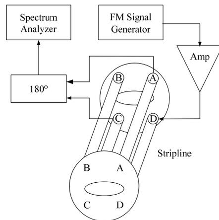
Figure 3: Layout of the tune measurement system at the SPS storage ring.
