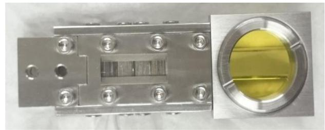
Figure 5: multi-slits stacked in a stainless steel holder.
