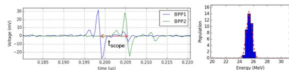
Figure 10: Energy measurement by TOF experiment.
