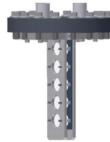
Figure 8: Carbon charge stripper foil mounted on ladder.
