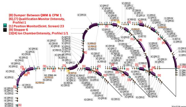
Figure 15: Layout and position of beam diagnostics in HEBT line.
