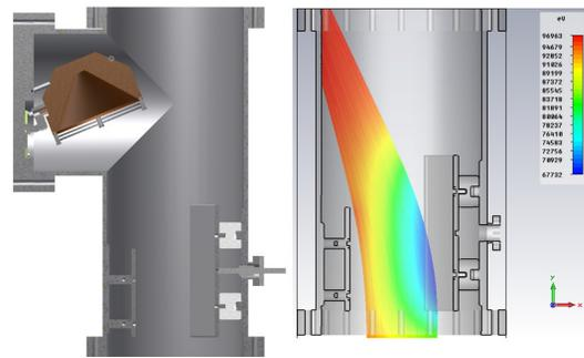
Figure 4: Electrostatic chopper in LEBT line.
