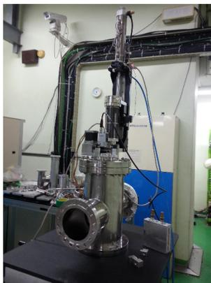
Figure 16: Scintillation screen monitor in synchrotron and HEBT line.
