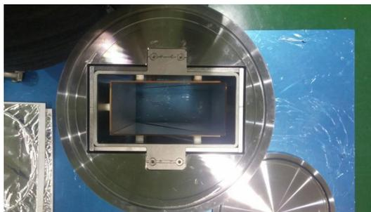
Figure 12: Linear-cut beam position monitor in synchrotron.
