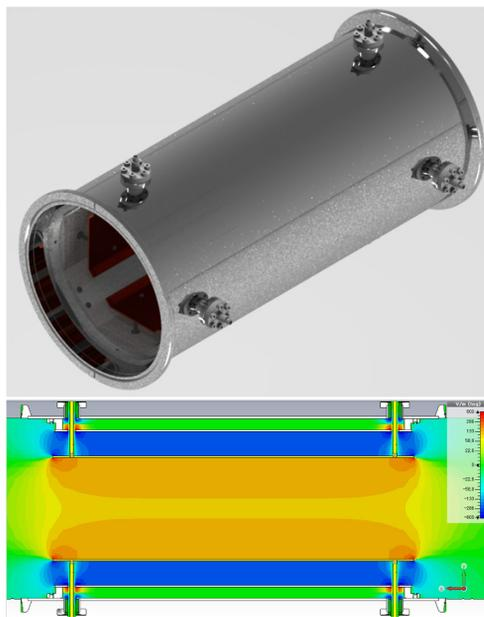
Figure 14: Stripline kicker in synchrotron.
