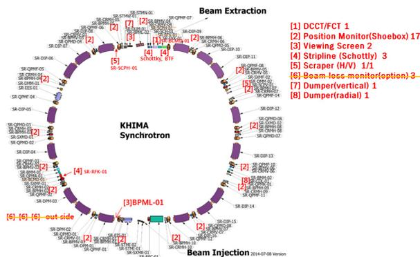
Figure 11: Layout and position of beam diagnostics in synchrotron.
