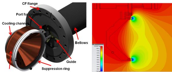
Figure 2: DC Faraday-cup and electric potential map of suppression ring in LEBT line.
