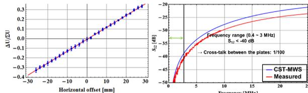
Figure 13: Measurement result of linearity and S-parameter of Linear-cut BPM.
