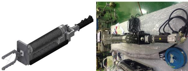
Figure 3: Wire-scanner in LEBT line.
