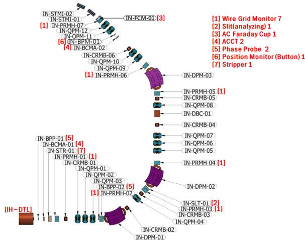
Figure 7: Layout and position of beam diagnostics in MEBT line.
