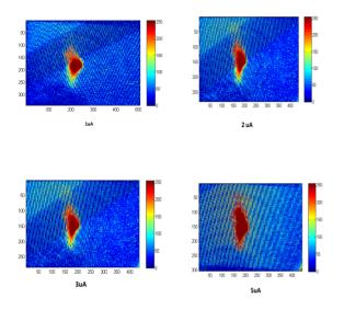
Figure 2: Beam shape at different beam intensities.
