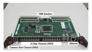
Figure 1: Developed VME/FPGA-based TDC module.
