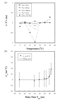
Figure 6: Variations (a) in the precision measurement depending on the set delay time within a dynamic range of 20 ms and (b) in the differential time difference between the measured and set delay time from a straight-line fitting within the same dynamic range.
