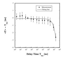
Figure 4: Variations in the time difference between the measured and set delay time with a dynamic range of 20 ms. Each solid point represents the average value over 5000 measurements and only the statistical error bars are plotted. The solid lines show a guide for the eyes only in a straight-line fitting.
