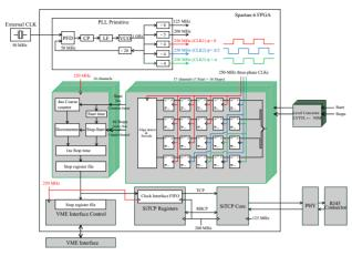
Figure 3: Schematic block diagram of the circuit architecture of the developed TDC. The meanings of the labels are detailed in text.
