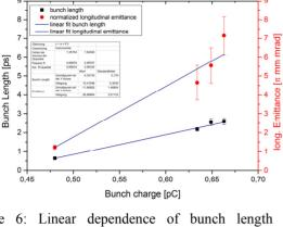
Figure 6: Linear dependence of bunch length and normalized long. emittance vs. bunch charge.
