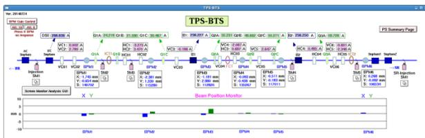
Figure 7: BTS GUI main page. BPM ADC data and detail configuration could be also accessed in the below pages.
