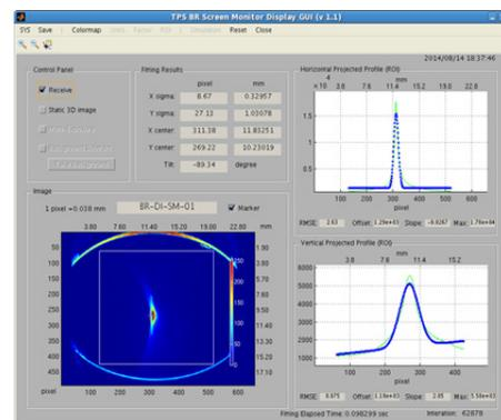
Figure 1: Beam profile at booster 1<sup>st</sup> screen monitor.
