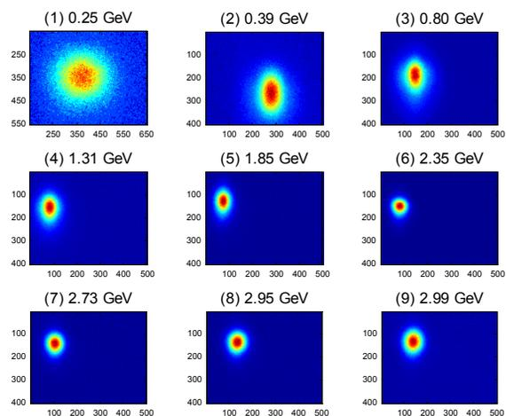
Figure 16: TPS booster synchrotron radiation profiles at varied energy ramping point, 1 pixel is around 9 μm.
