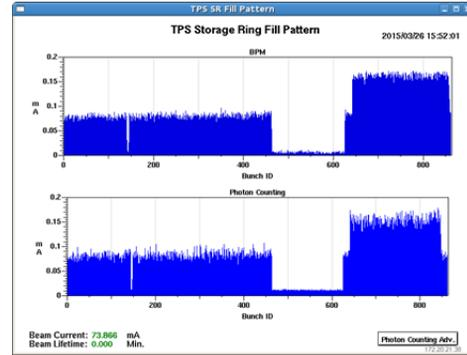
Figure 5: Filling patterns of the storage ring are measured from BPM button (upper) and TCSPC (lower).
