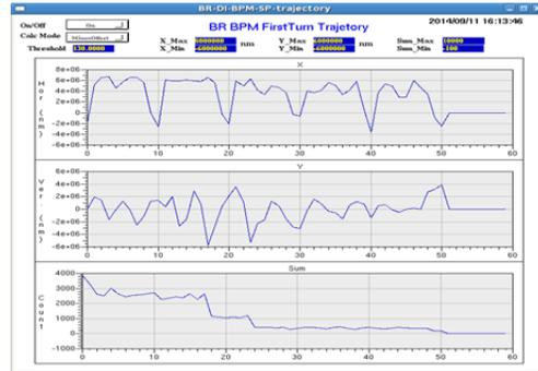
Figure 9: First turn horizontal, vertical trajectory and sum along 60 BPMs of booster. Horizontal trajectory shape like dispersion and it indicates the injection beam energy is higher that dipole current settings.
