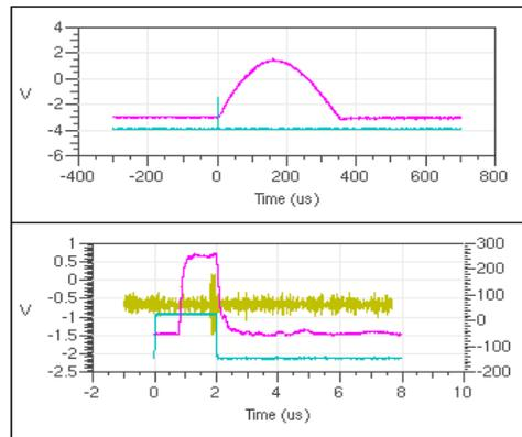
Figure 8: The upper plot is septum waveform (pink) and its trigger (blue). The below plot is kicker waveform, its trigger and ADC data of booster 1<sup>st</sup> BPM button D (yellow) located between the pulse of kicker waveform.
