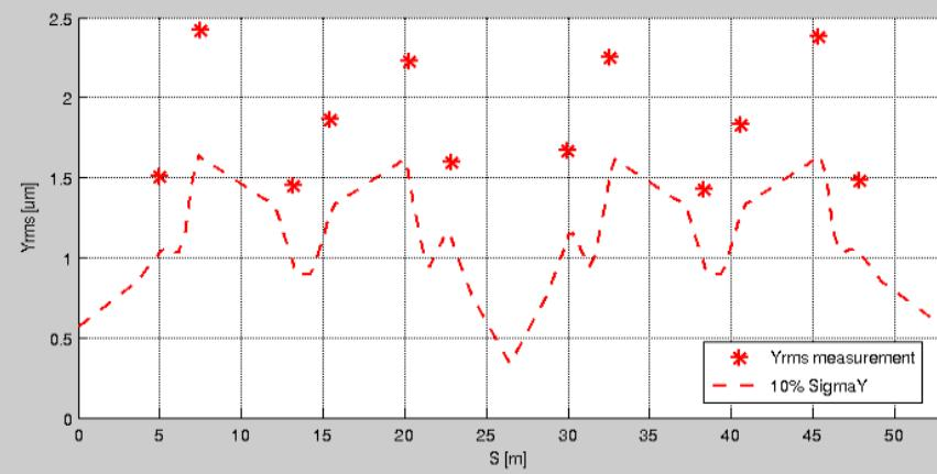
Xrms, Yrms integrated from psd in the range of [10,1000]Hz
