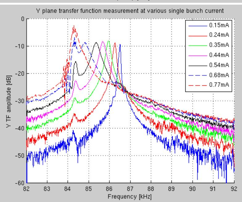
Vertical plane tune spectrum at different single bunch current looks like TMCI
