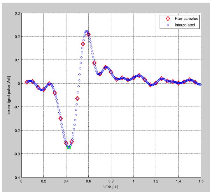
2014-Jul-13 data, use FPM to measure synchronous phase at various Vrf, keep the current same and filling pattern.  $I = 2.1\text{mA}$ , 20-bunches in one bunch train.
