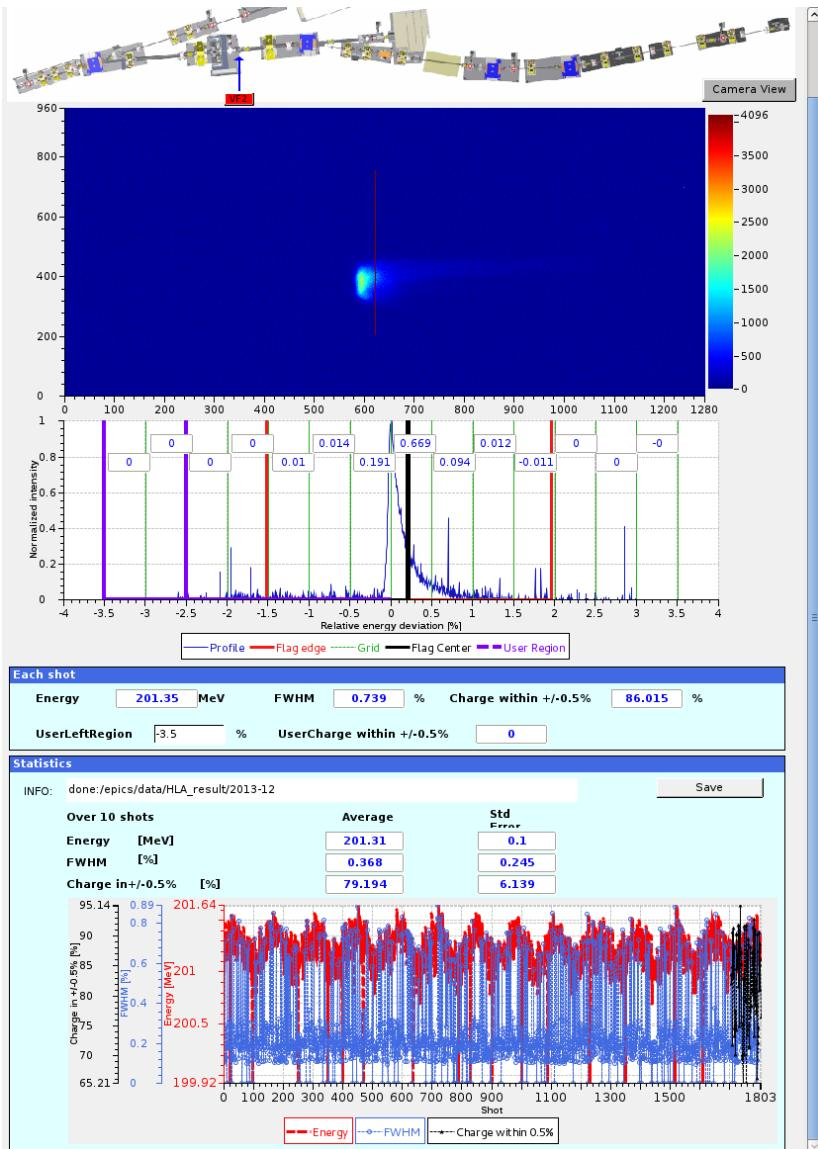
Energy jitter and energy spread measurement, using LtB VF2.
