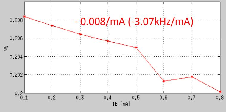
$$\Delta Q_\beta = \frac{I_b T_0}{4\pi E / e} \langle \beta \rangle k_{\perp total} = \frac{I_b T_0}{4\pi E / e} \sum_j \beta_j k_{\perp j}$$
