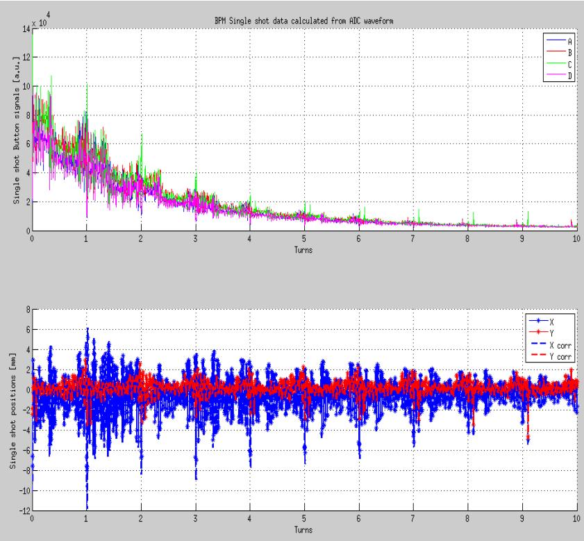
x/y position nonlinearity corrected using 5<sup>th</sup> order polynomial
