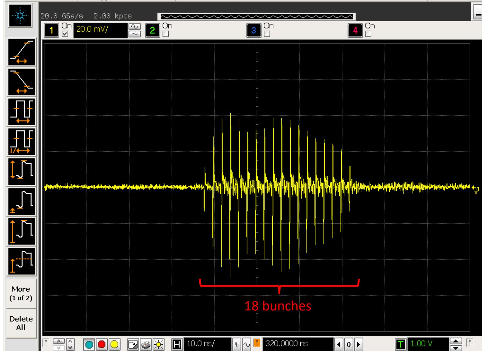
Stored beam  $\sim$ 1.58mA. 18 bunches with e-Gun pulse width set to 35ns
