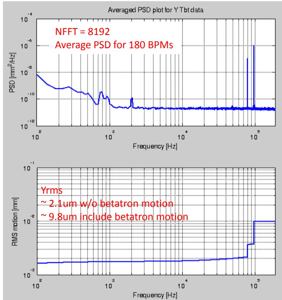
10kHz FA data characterize the lower frequency (< kHz) beam motions
