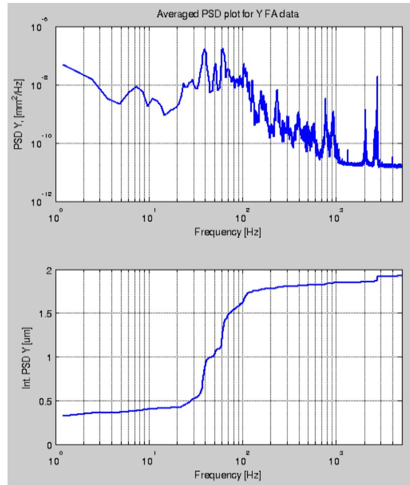
NFFT = 8192, PSD spectrum averaged for three blocks of FFT
