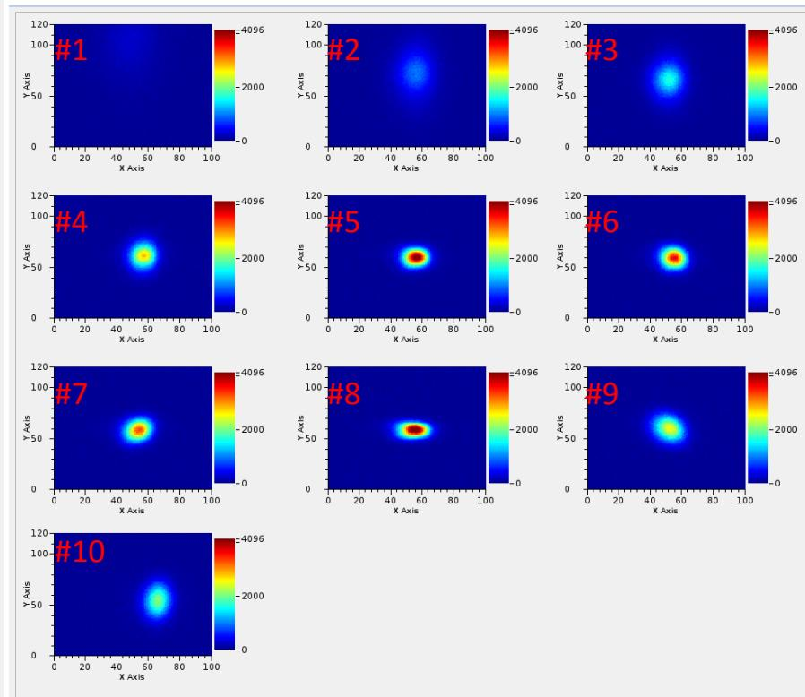
10 burst images acquired on the same booster ramp cycle, separate by 40ms
