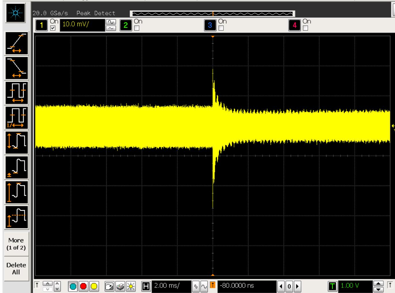
Captured on Apr-11, after Booster energy and SR RF phase adjusted, didn't see the dip on BPM raw button SUM signal.
