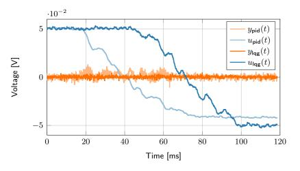
Effects measurable with PID controller but not with LQG.
