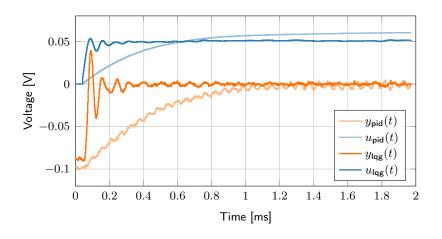
The model based controller reaches the steady state faster ...
