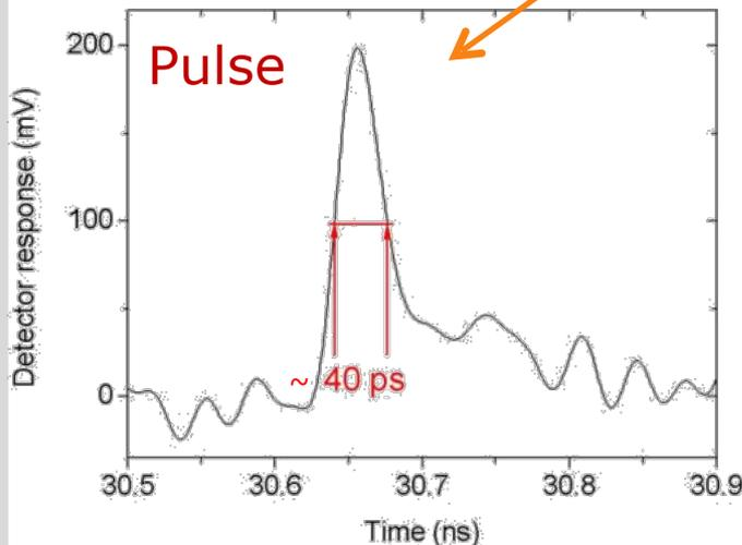
Pulse measured with a real-time oscilloscope (bandwidth 60GHz)
