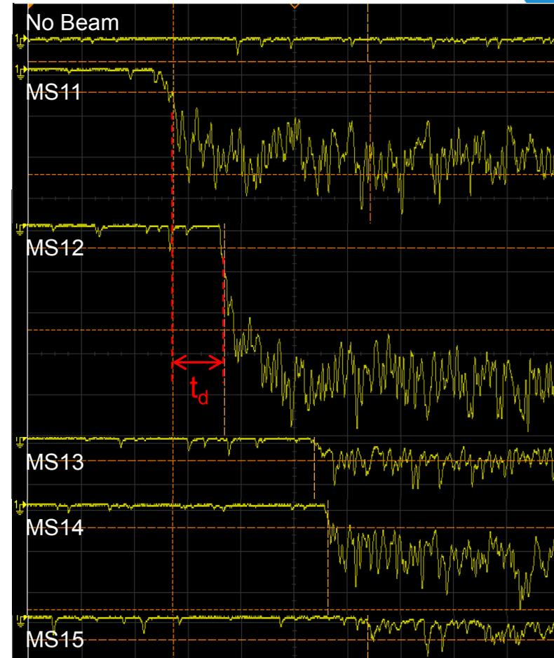
We can estimate the beam-loss point along the circumference by analyzing the time structure of the output signal.
