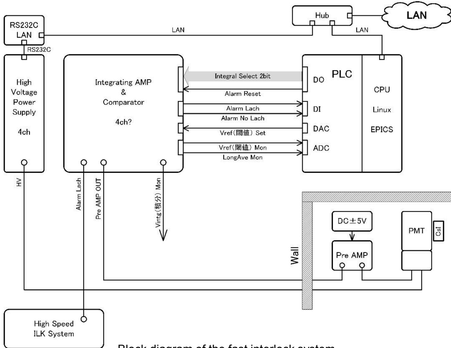
Block diagram of the fast interlock system
