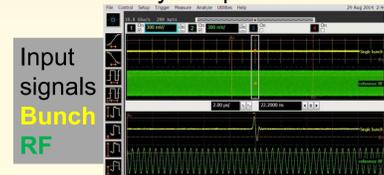
To simulate the single bunch selector, a generator with two outputs at the same frequency is used. The first output corresponds to the RF frequency (green curve) and the second (yellow curve) to the pulse.
