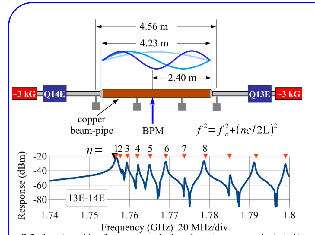
Reflections at transitions from copper to aluminum beam-pipe are present due to the higher cutoff frequency of the aluminum extrusion. In this case, the resonant series matches the calculation based on the cutoff frequency and the 4.23 m length of the copper section.
