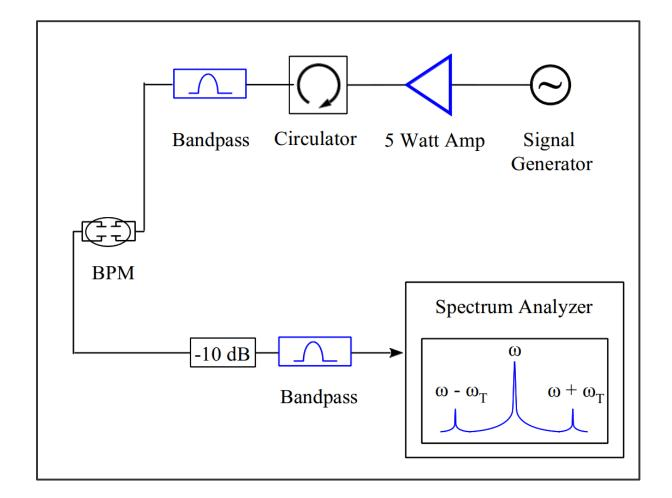
Hardware: The drive and receive signals are routed to/from three locations in the 13-15E sector of CESR (upper). The instruments needed to make an EC density measurement are shown in the lower part of the figure.
