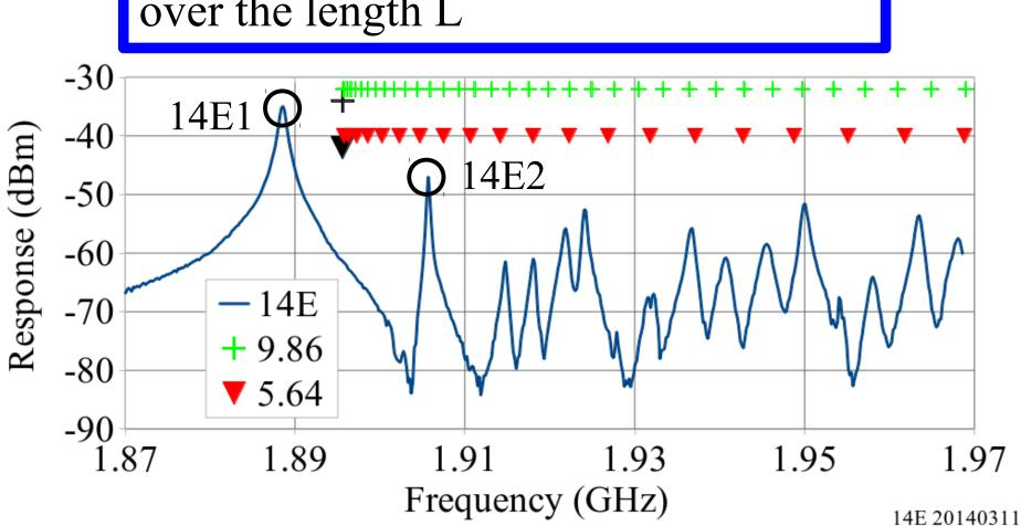
With drive/receive at 14E, a single length L does not give the observed resonant series. As a result it is difficult to know what length of vacuum chamber the standing waves occupy. The series for L = 9.86 and 5.64 are shown.
