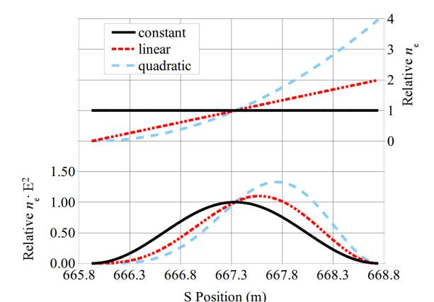
A non-linear change in EC density with position will affect the integral of Eq. 1. We make the approximation that the EC density is proportional to the synchrotron light in order to calculate a compensation for this effect so that the density at the resonance center can be calculated.
