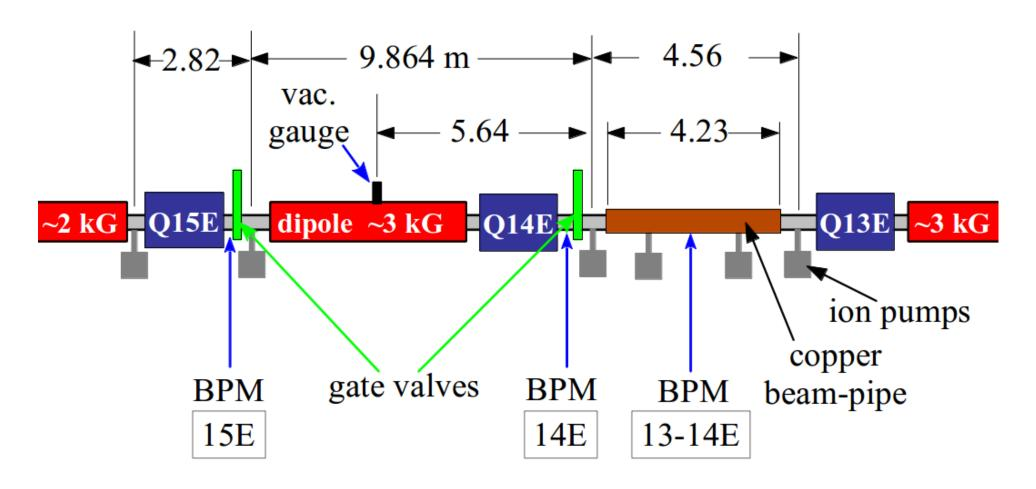
Dimensions in the 13-15E sector are used to calculate the expected resonant frequencies. The model is a shorted section of waveguide, with reflections produced at the longitudinal slots at ion pumps or transitions in beam-pipe geometry. The response at drive points 13-14E and 15E give a reasonable match to the measured response, but at 14E (right) the resonant series is not as simple.
