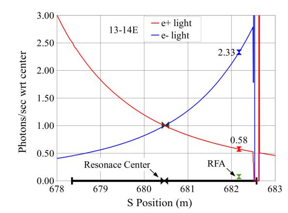
The EC density at CESR is generated primarily by synchrotron radiation. The plot above shows that synchrotron radiation changes by a factor of 5 over the resonance length at 13-14E.
