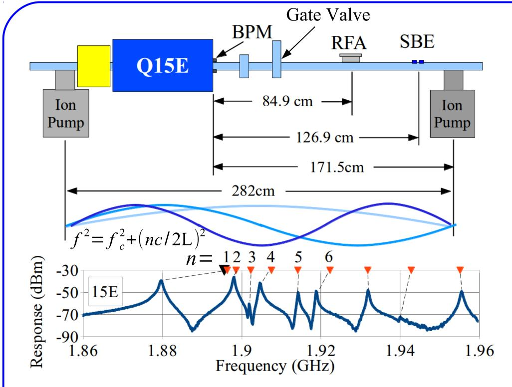
**Reflections at ion pumps** produce resonances in the beam-pipe, with the response measured at 15E shown above. The peaks do not follow a resonant series very well. It is suspected that the larger volume in the gate valve pulls the some of the resonant frequencies lower.
