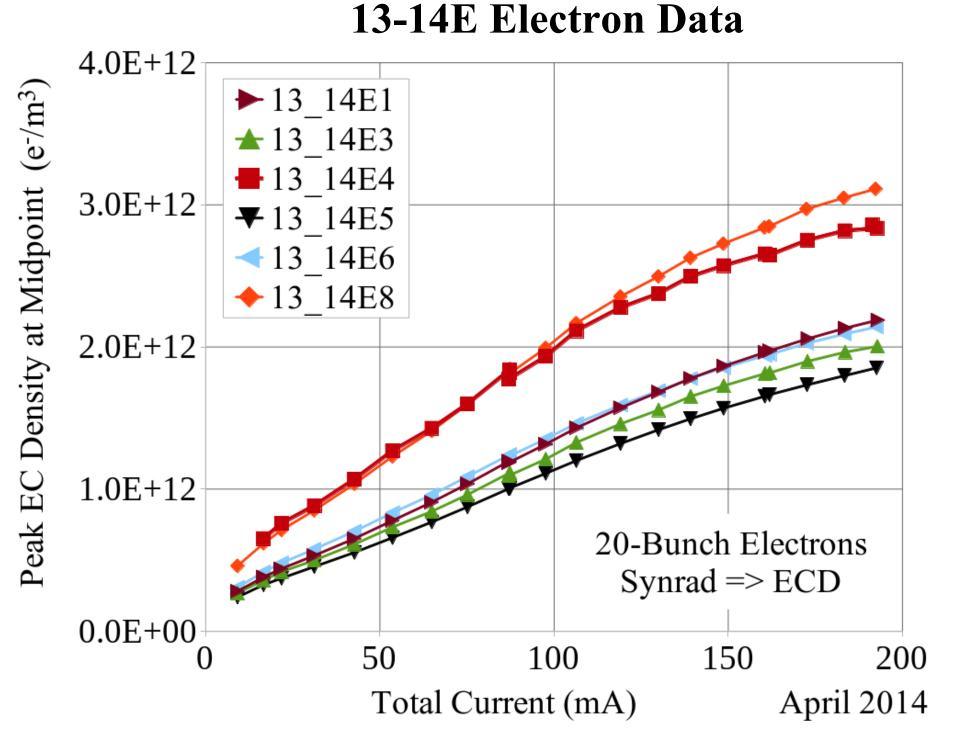
The 13-14E copper chamber shows a fairly linear EC density with beam current for both positron and electron beams. The EC density obtained for the different resonances varies by more than 50%. This suggests that there is something unaccounted for in the calculation of EC density.
