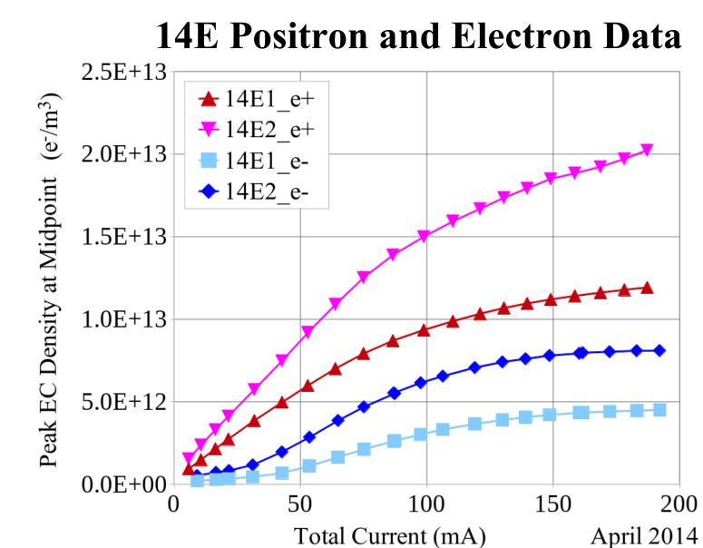
At 14E the two lowest resonances were used, 14E1 and 14E2. For both positrons and electrons, the EC density measured by 14E1 and 14E2 differ by about a factor of two. This needs further explanation.
