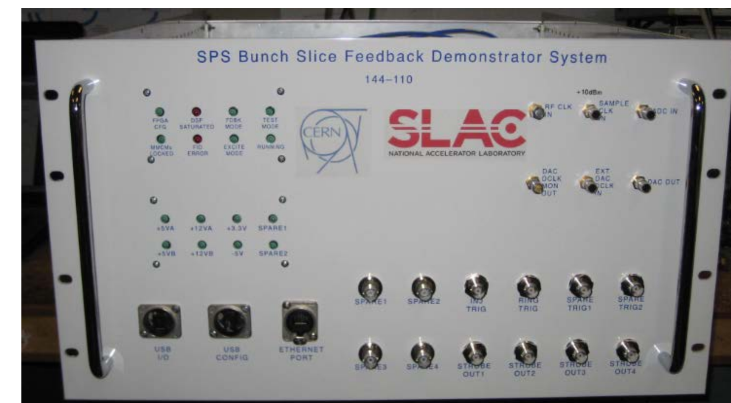
System Chassis: all boards, cabling, cooling & power supply are packaged inside
