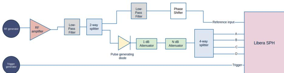
Figure 1: Block diagram of the measurement setup used for measurements with centred beam conditions.
