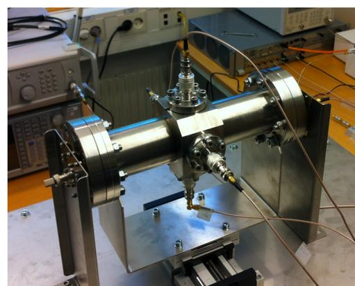
Figure 6: BPM test-bench designed and assembled at ESS.
