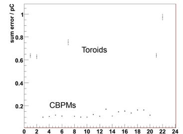
Figure 11: Sum of statistical and systematic errors of charge monitor correlation at FLASH2 at a charge of about 100 pC, with active automatic gain control of the CBPMs, ordered according beam direction.
