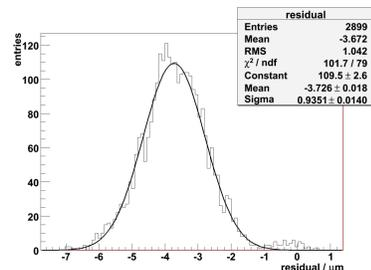
Figure 6: Residuals at a mean beam offset of 0.46 mm and charge 240 pC with Gaussian fit.
