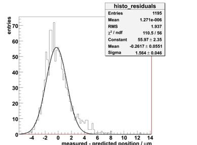
Figure 12: Difference between expected and measured position with Gaussian fit of a CBPM with monitor number 4 for position error calculation at the horizontal plane.
