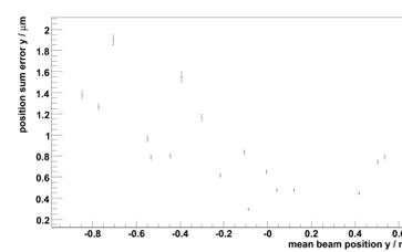
Figure 14: Sum error of CBPM correlation measurement at FLASH2 at the vertical plane with a charge of about 100 pC as a function of mean beam position.
