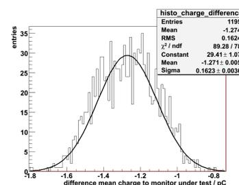
Figure 10: Difference between mean charge value to the monitor under test: here CBPM with the monitor number 19 with Gaussian fit; charge of about 100 pC.
