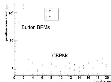
Figure 13: Sum error of BPM correlation at FLASH2 in both transverse planes for a charge of about 100 pC.
