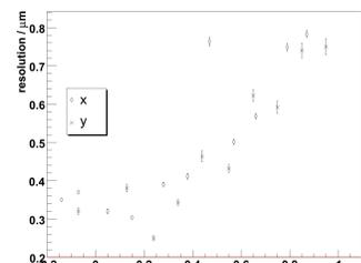
Figure 7: Resolutions of the undulator CBPMs at FLASH1 for different mean beam offsets in x and y for a charge of about 240 pC.
