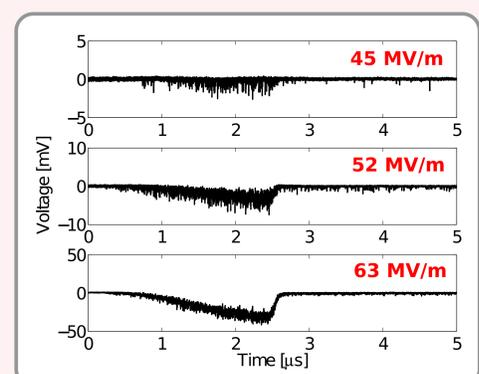
At PHIL, the FBLM can be used to condition the dark current (detection limit below 1 pC).
