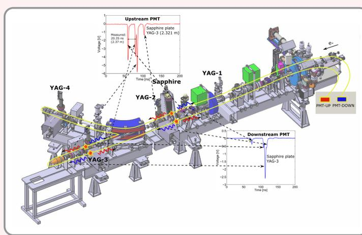
The fiber of 25 meters was installed alongside the vacuum chamber to cover continuously the total length of the photoinjector from both sides.
