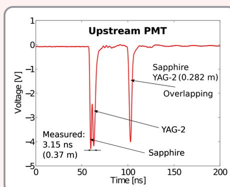
Two peaks spaced by  $\sim 3$  ns defines time resolution of the FBLM.
