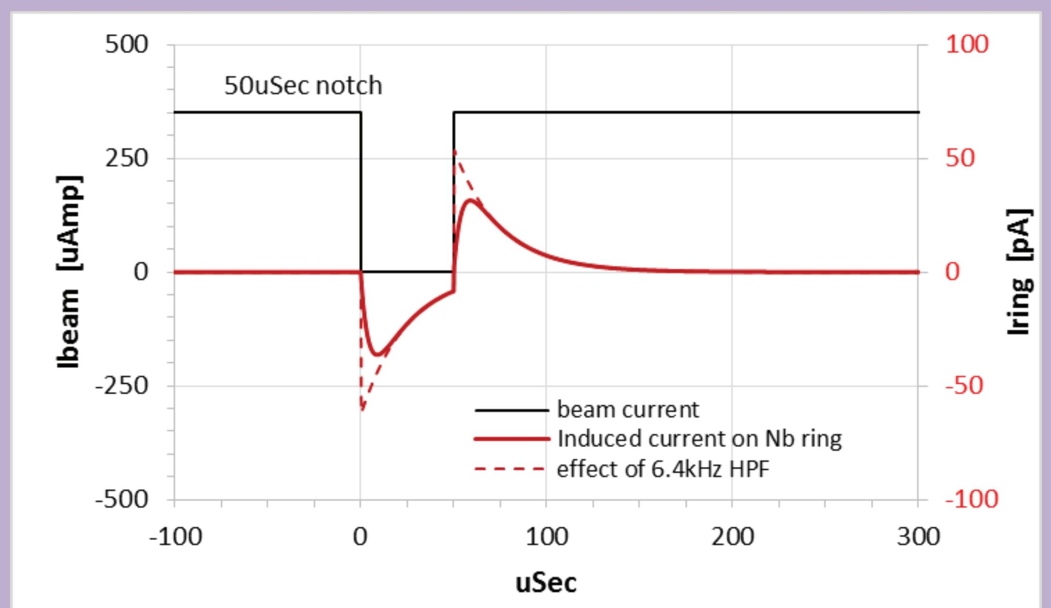
The  $I_{ring} / I_{notch}$  could be modeled as a 6.4kHz high pass filter (HPF). Combined with the 33kHz LPF that we plan to use, the final induced current will be ~33pA. Compared with LMR desired detection limit  $100 \pm 50 \text{ pA}$ , it is still tolerable. It, however, brings some fake background when we take the samples in the notch for background subtraction. Integration in an extended time could help.
