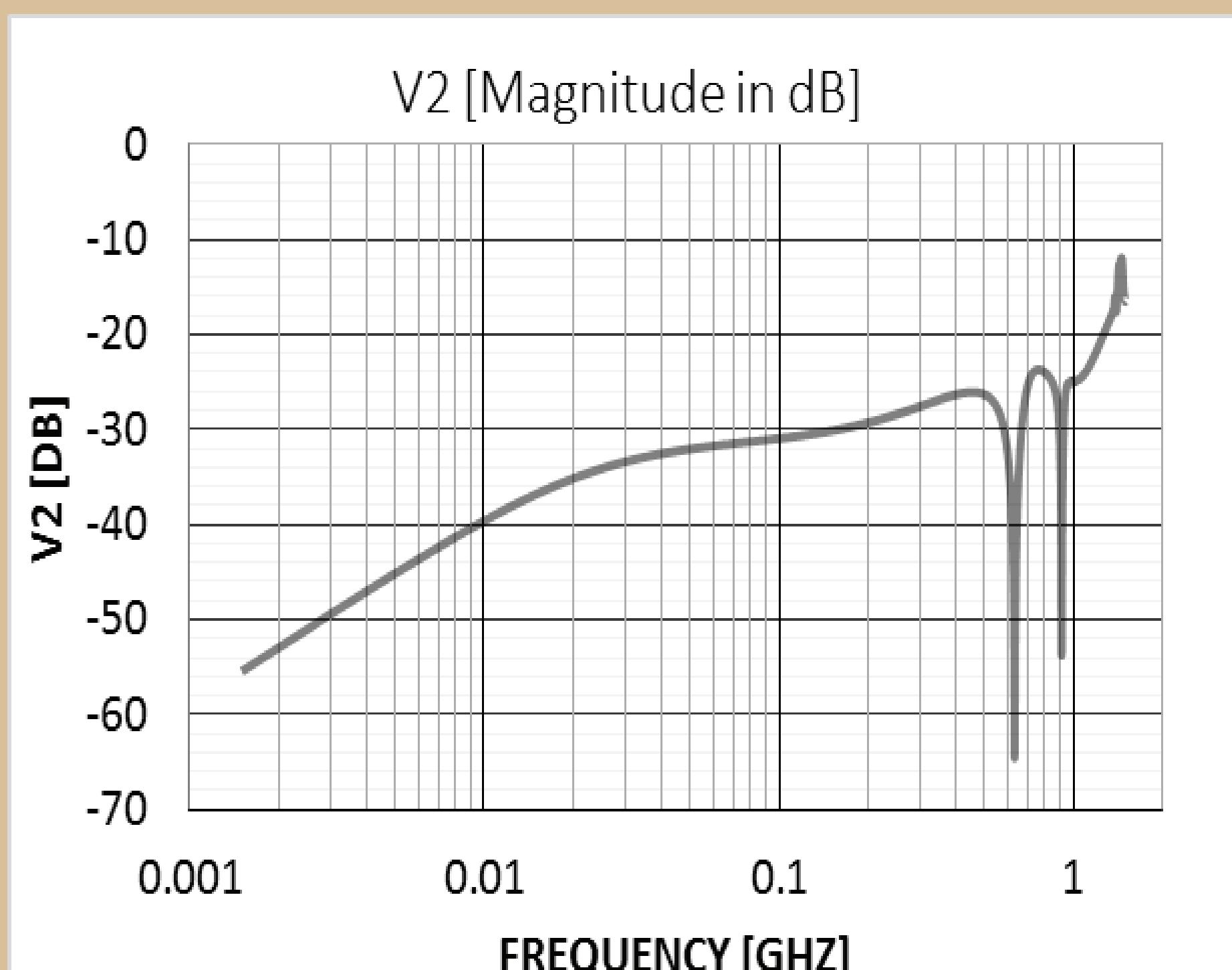
Comparison of output voltages with different structures of LMR. Different colors correspond to a) only niobium intercept, b) adding grounded copper plates, c) adding washers and bolts.
