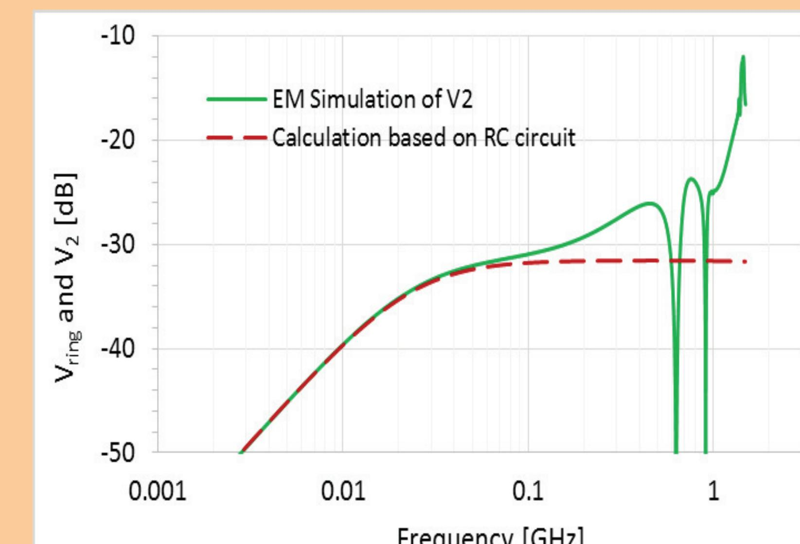
For Niobium intercept only, C is 3 pF. Corner frequency of RC circuit is 1.2 GHz.
