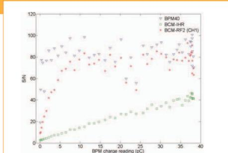
The newly developed Turbo ICT makes use of several ferrites whose signals are combined to reduce the noise floor. A signal-to-noise ratio of more than 60 is obtained for the SwissFEL charge range of 10 to 200 pC. The measurement shown above is limited by the charge variations in the beam.
