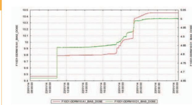
On-line measurement of dose rate with a RadFET, during the undulator experiment
