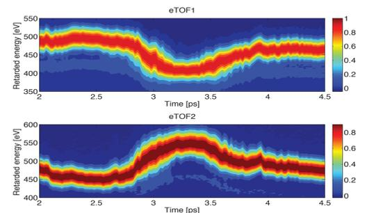
The normalized signal from the THz scan for 10 keV photon beam. The spectrum of the photoelectrons changes during the scan in accordance to the shape of the vector potential.
