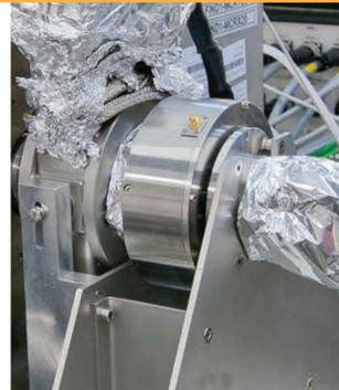
This monitor will be used for a beam-based calibration of the cavity BPMs.
