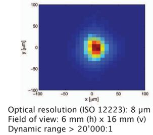
Optical resolution (ISO 12223): 8  $\mu\text{m}$
