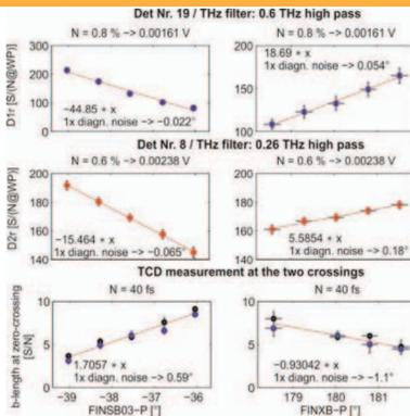
Experimental results on varying the compression phase (FINSB03-P) and the phase of the fourth harmonic (FINXB-P) for a bunch length of roughly 260 fs and a bunch charge of 20.5 pC (energy: 200 MeV). Top two rows: BCM signals integrated in the two spectral ranges, bottom row: bunch length measured by the transverse deflecting cavity.
