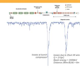
A longitudinal loss monitor, consisting of a fiber optic cable installed along the beamline, allows determining the location of beam losses
