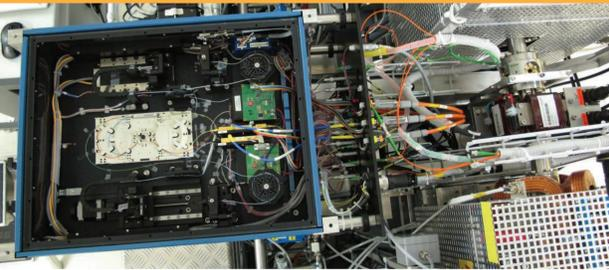
Improvements 2014: button pick-ups equipped with 40 GHz vacuum feedthroughs, EOMs with 33 GHz bandwidth (40 Gs/s) and small half-wave voltage (4.6 V), DC-offset DAC, improved photoreceiver. Intrinsic resolution: 10 fs - 13 fs @ 90...200 pC, 13 fs - 40 fs @ 20...90 pC.
