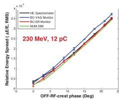
Comparison of energy spread measurements using the SR imager with measurements using scintillators in the bunch compressor as well as just before the beam dump, and with a numerical model
