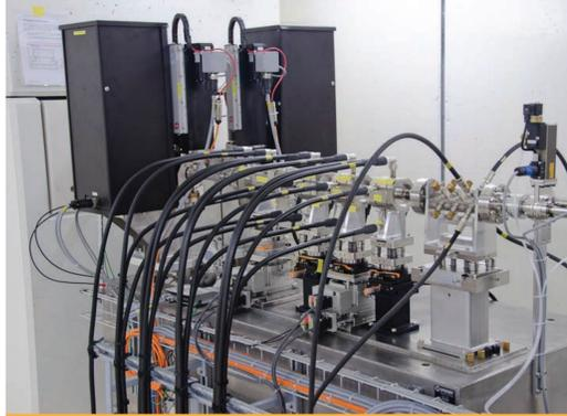
SwissFEL BPM16 position resolution measurement: difference between SwissFEL and XFEL.EU (extrapolated) BPM position reading
