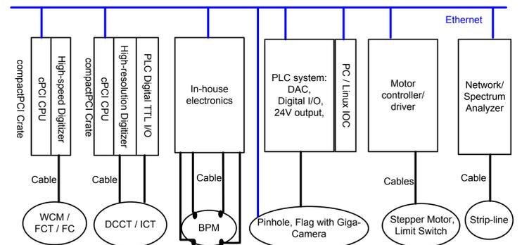
Figure 3: Diagnostics Controls Interfaces
