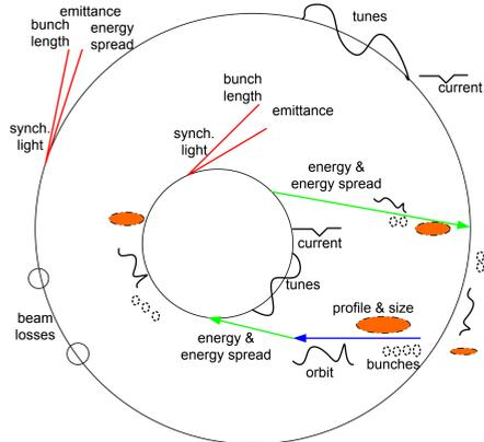
Figure 1: Beam Parameters Measured at NSLS-II
