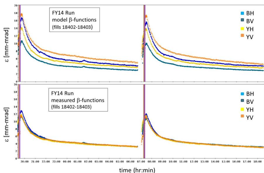
Figure 4: Evolution of the transverse beam emittances with 3D stochastic cooling [9] during the FY14 RHIC Run derived from the IPM profile measurements in all 4 planes (horizontal and vertical in the Blue and Yellow Rings) during two physics stores derived using model beta functions (top) and, for the same two stores, using beta functions interpolated from measurements from nearby beam position monitors (bottom).
