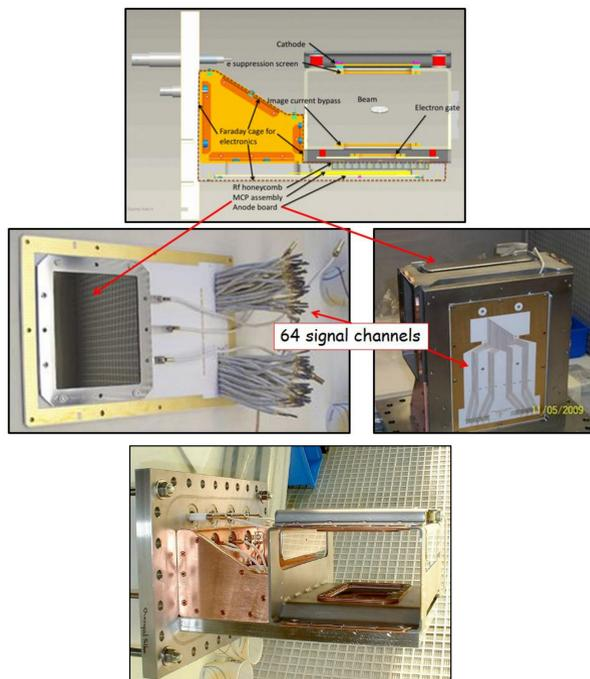
Figure 1: Conceptual view (top) and photographs (bottom) of new RHIC IPM [5]. The MCP (left) dimensions are 8 cm by 10 cm. The signals from the MCP are collected by the 64-channel anode board (right) and read out through the ceramic-beaded wires (left).
