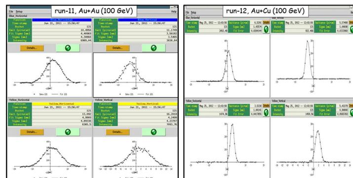
Figure 3: Example beam profile measurements before (left) and after (right) implementation of IPM offset and gain corrections. Shown in the top row are the Blue ring horizontal (left) and vertical (right) profiles and in the bottom row the Yellow ring horizontal (left) and vertical (right) profiles.
