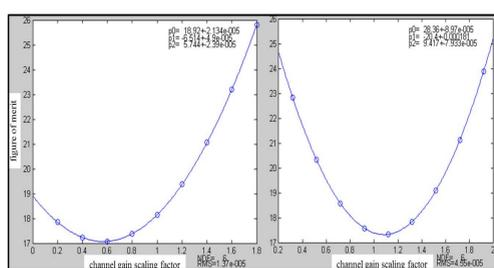
Figure 2: Example polynomial fits to figure of merit,  $\langle \chi^2 \rangle$ , versus channel gain scaling factor for two different IPM channels.
