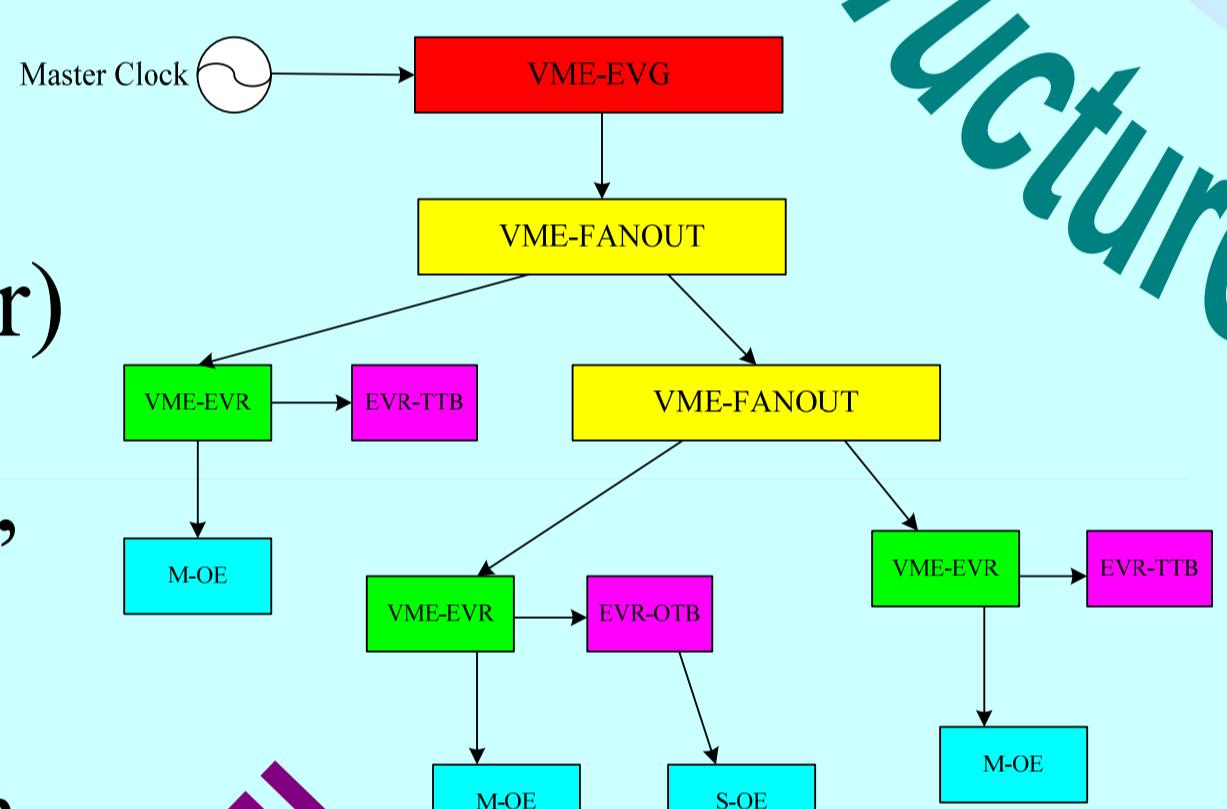
SINAP v2 timing system adopts similar topology based on fiber-optic network as well, but communication mode upgrades from simplex to duplex, which means that we could conduct deterministic data transfer and event distribution at the same time.
