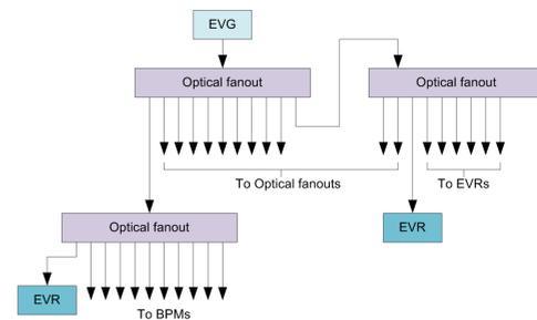
**Figure 2.** Optical event distribution block diagram. Events are transmitted from the EVG via 1:11 optical fanouts to EVRs and clients with embedded EVRs (i.e. BPMs).
