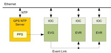
**Figure 1.** Timestamping block diagram. The timing IOCs get GPS time from the NTP server via Ethernet at boot time. The server also sends a GPS-locked Pulse Per Second (PPS) trigger to the EVG.
