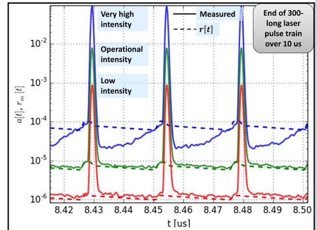
**LHC Data:** The figure shows raw data from Beam 2 during fill #3005 in 2012, and corrected data (photon + background rate). The raw data shows a "baseline" variation between main bunches by more than one order of magnitude, caused by afterpulsing. Corrected, the baseline is flattened and the satellite/ghost bunch structure is resolved.
