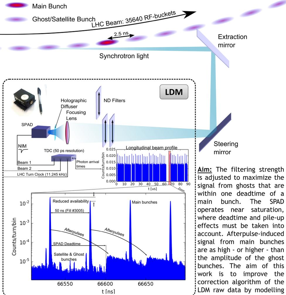
**Aim:** The filtering strength is adjusted to maximize the signal from ghosts that are within one deadtime of a main bunch. The SPAD operates near saturation, where deadtime and pile-up effects must be taken into account. Afterpulse-induced signal from main bunches are as high - or higher - than the amplitude of the ghost bunches. The aim of this work is to improve the correction algorithm of the LDM raw data by modelling and removing afterpulses from raw data.
