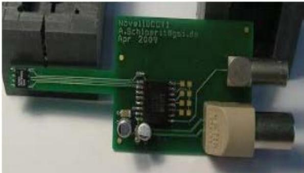
Figure 5: GMR Test PCB.
