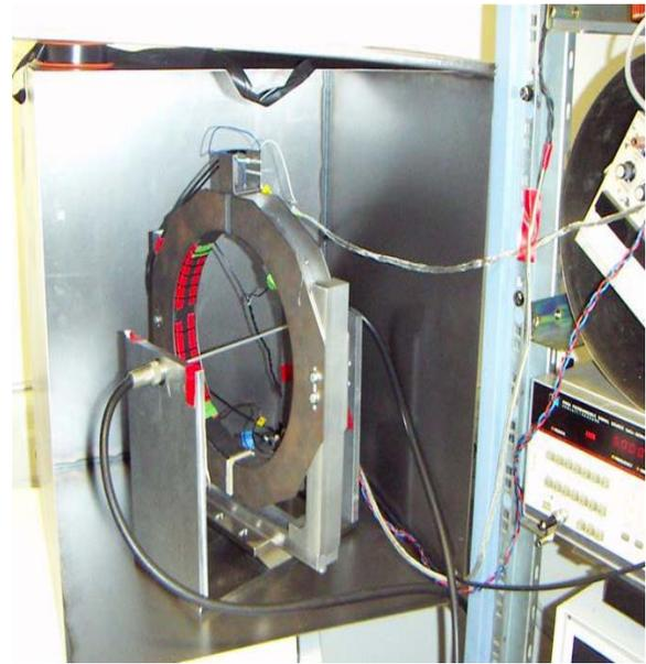
Figure 10: NDCCT Test Setup.
