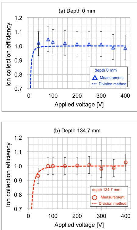
Figure 5: Comparisons of the saturation curves between measurements with the position error and calculation results obtained by using the division method. This is the same comparison represented by the Figure 4 (b). The error bar indicates the variation range with variation of the detector center position with  $(x, y) = (\pm 0.1, 0.0)$  mm.
