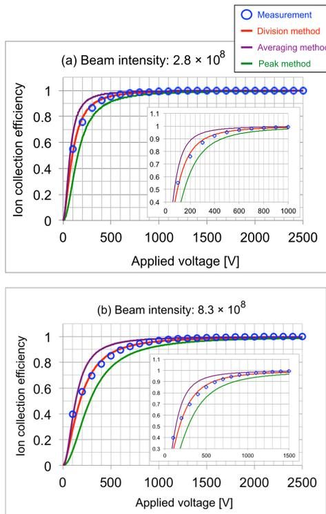
Figure 3: Comparisons of the saturation curves between measurements and calculation results obtained by using different calculation methods for the parallel plate ionization chamber.
