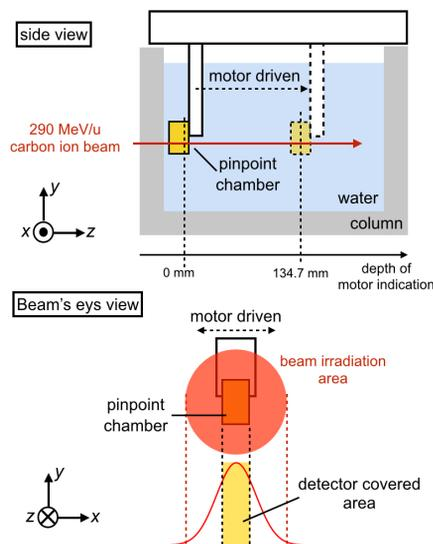
Figure 2: Experimental arrangement using a cylindrical pinpoint ionization chamber.
