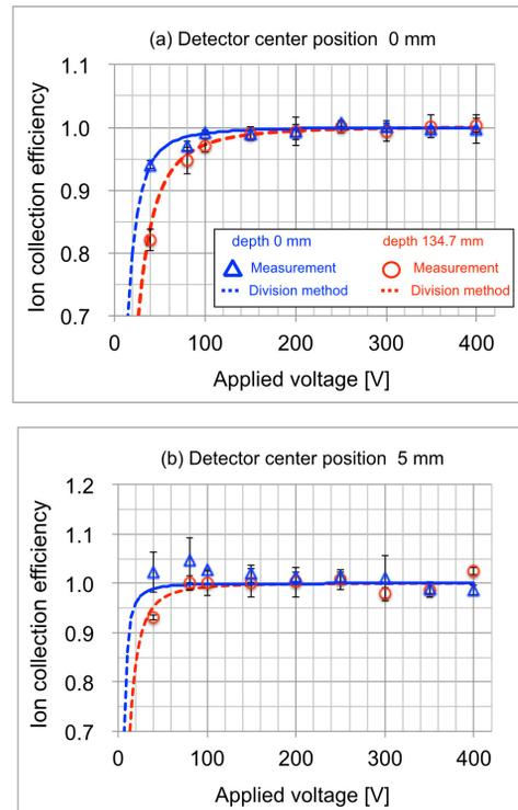
Figure 4: Comparisons of the saturation curves between measurements and calculation results obtained by using the division method for the cylindrical pinpoint ionization chamber.
