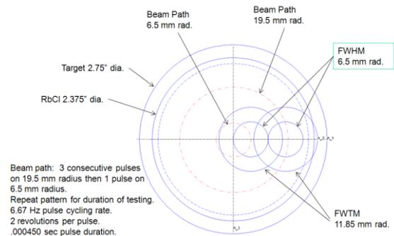
Figure 1: Diagram of circular raster pattern on target.
