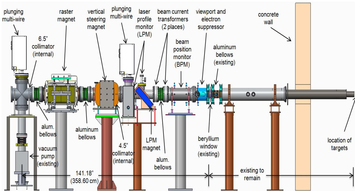
Figure 2: New BLIP beam-line layout.
