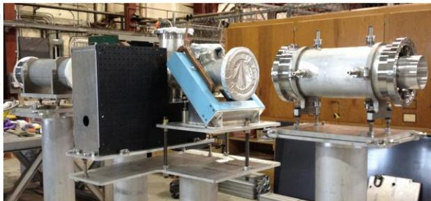
Figure 7: Beginning of mock-up of new BLIP beamline section including from left to right, the dummy raster magnet spool piece, the LPM with optics box (black side) and detector magnet (blue), and the BPM. Beam direction is left to right.
