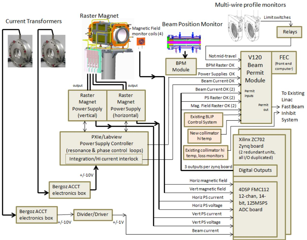
Figure 6: BLIP beam interlock system block diagram.
