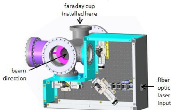
Figure 4: BLIP LPM chamber and optics/motor assembly.
