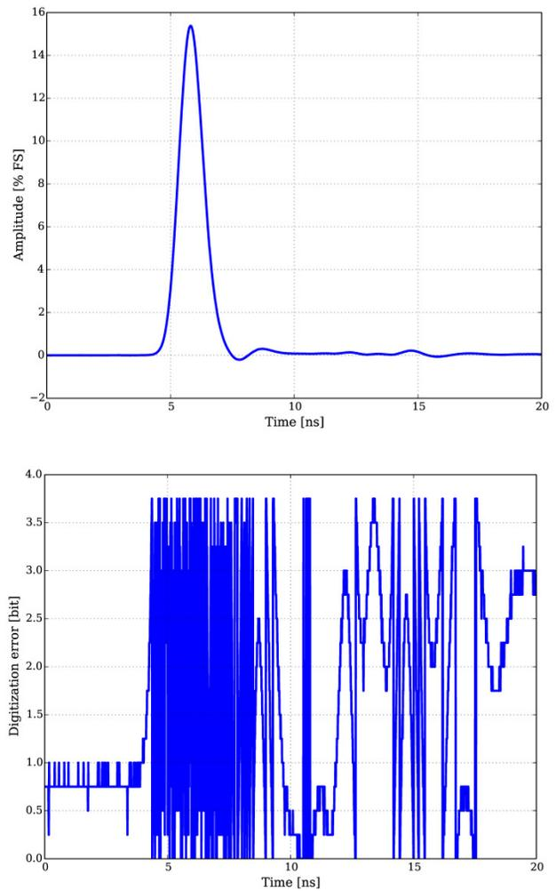
Figure 5: 8-bit dataset computed from the 12-bit dataset for the 1.2 ns pulse (top). Bits of error per sample of the 8-bit dataset obtained by comparing it to the 12-bit data (bottom).
