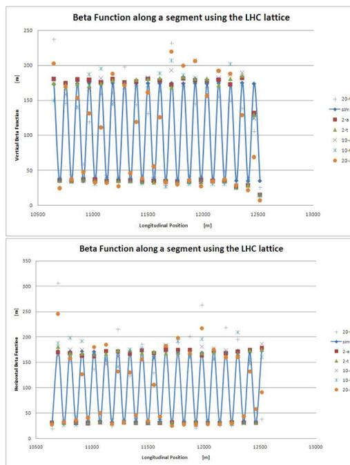
Figure 4: Beta Functions for a sector of the LHC lattice , without and with noise for 2, 10 and 20 degrees of deviation.
