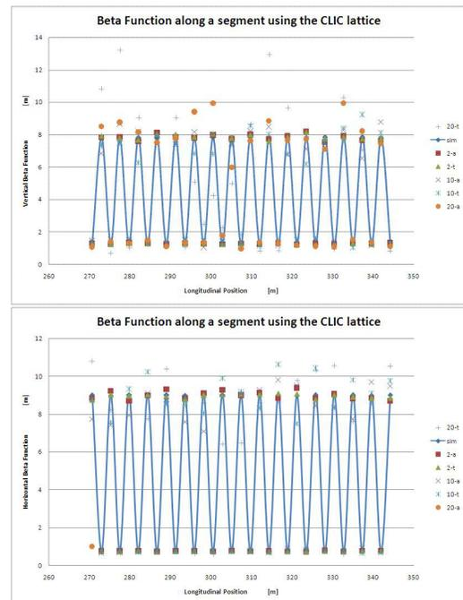
Figure 3: Beta Functions for a sector of the CLIC lattice, without and with noise for 2, 10 and 20 degrees of deviation.
