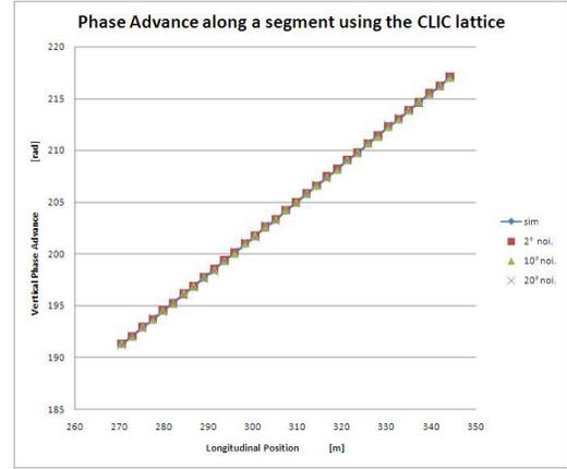
Figure 1: Phase Advances for a sector of the CLIC lattice, without and with noise for 2, 10 and 20 degrees of deviation, for the Y plane.
