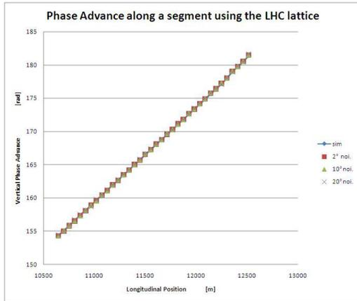
Figure 2: Phase Advances for a sector of LHC lattice, without noise and with noise of 2, 10 and 20 degrees.
