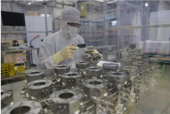
Figure 2: Assembly of button BPMs in cleanroom environment.
