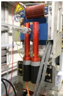
Figure 8: Pair of type X-FEL type BLMs installed in the FLASH2 beamline.
