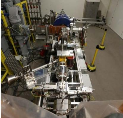
Figure 10: RF gun with first about 1.5 m long beamline installed in the injector building.
