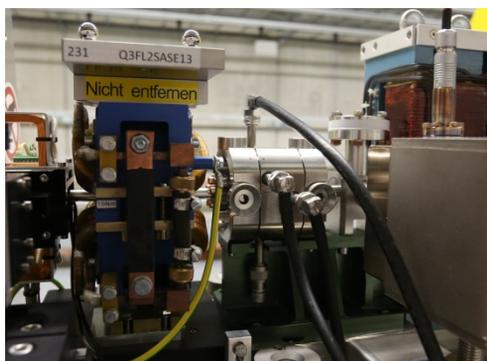
Figure 6: XFEL cavity BPM of the Undulator type installed in an Undulator intersection of the FLASH2 beamline.
