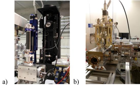
Figure 7: E-XFEL screen station and wire scanner.
