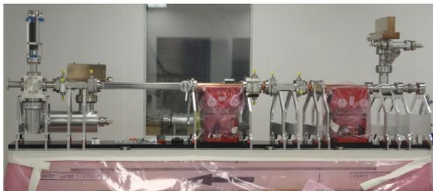
Figure 5: XFEL girder with two 40.5 mm cavity BPMs during assembly in the clean room.
