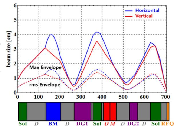
Figure 3: The beam optics simulation results using TRANSPORT code.
