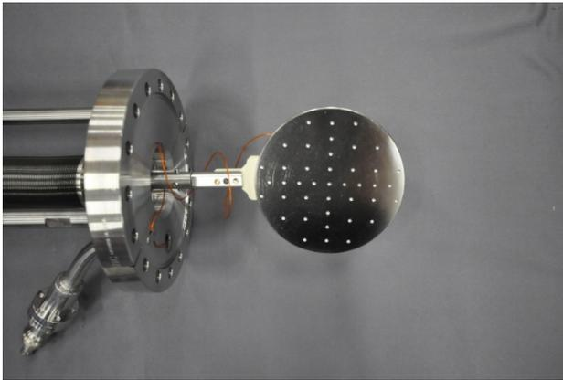
Figure 5: The photo of view screen with pin holes.
