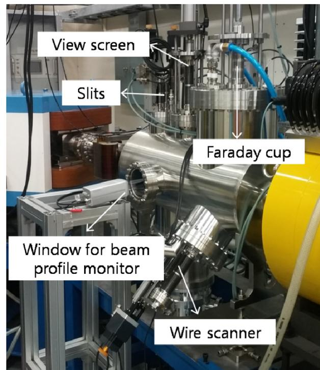
Figure 4: The photo of diagnostic chamber with measuring devices.
