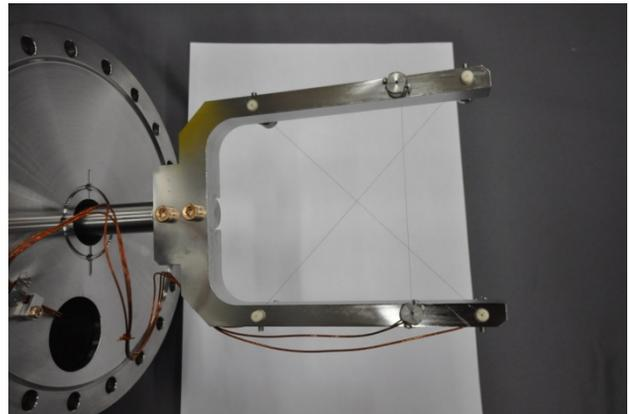
Figure 8: The photo of wire scanner with three wire.
