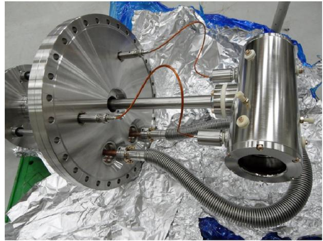
Figure 7: The photo of the fabricated faraday cup.
