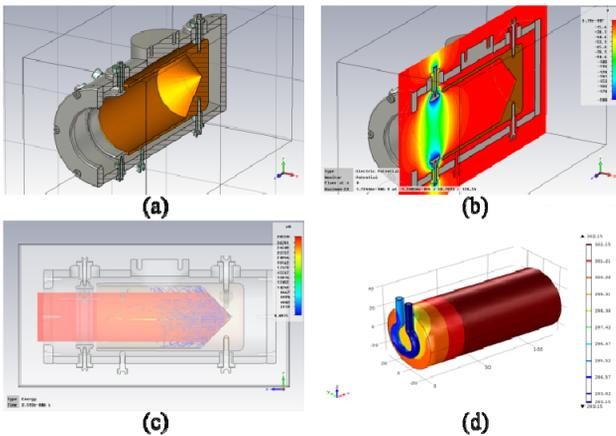
Figure 6: The simulation results of Faraday cup 3D model (a), potential distribution (b), secondary electron tracking (c), temperature distribution with cooling channel (d).
