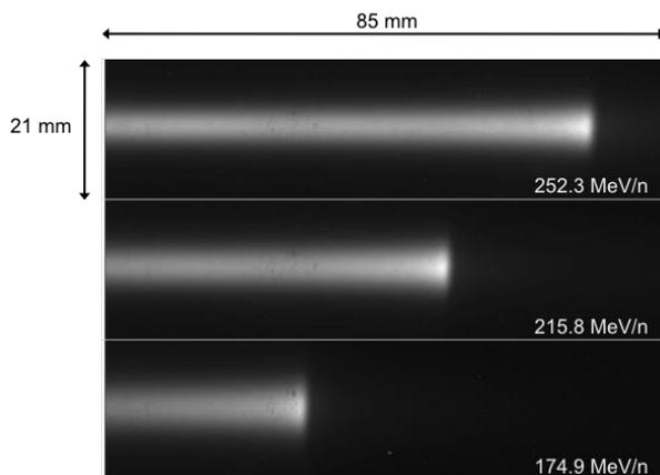
Figure 4: Example of the depth brightness distribution acquired with CCD camera.
