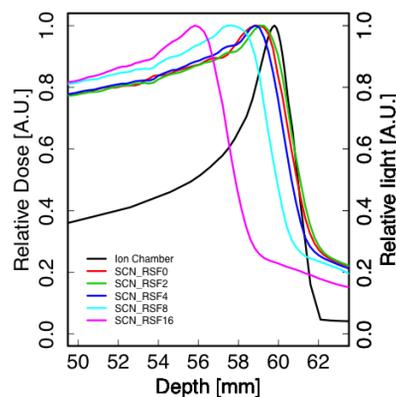
Figure 5: Comparison between the reference depth dose measured by ionization chamber and relative light output shifted by RSF.
