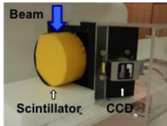
Figure 1: Layout of the scintillator and CCD system.
