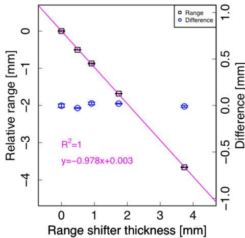
Figure 6: Comparison of the relative range with range shifter thickness.
