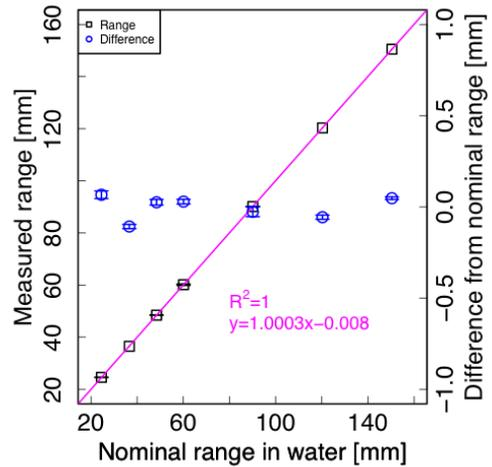
Figure 7: Measured range using DOG method and difference from nominal range.
