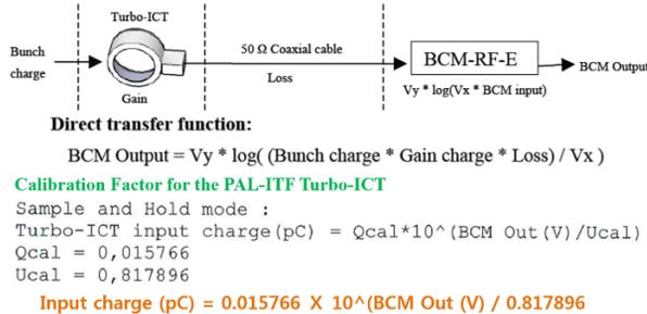
Figure 13: Calculation formula of Turbo-ICT charge amount.
