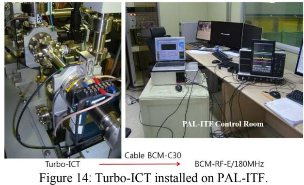
Figure 14: Turbo-ICT installed on PAL-ITF.
