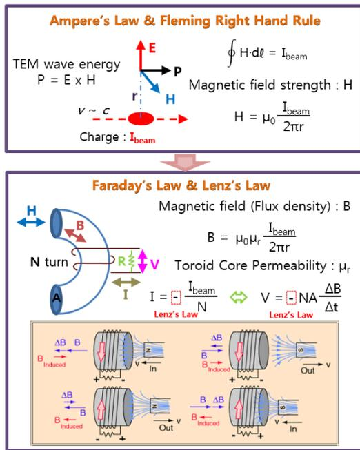
Figure 7: Physical principle of ICT.
